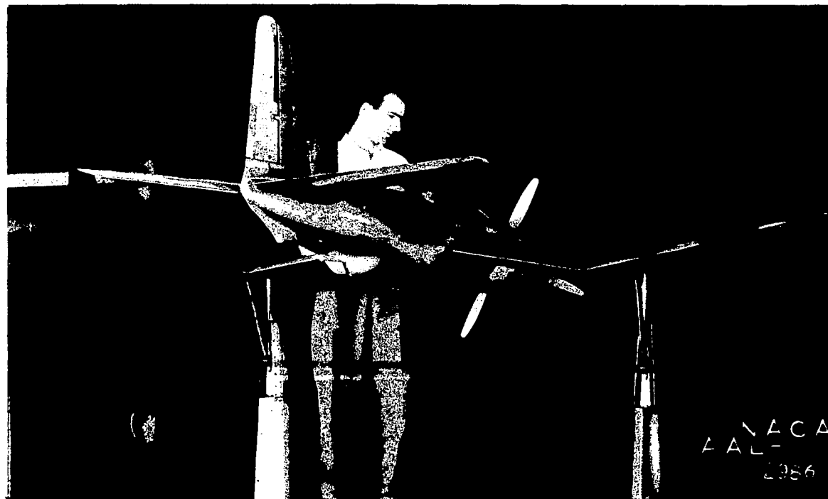
Figure 2.- A 3/16-scale model of the Douglas XSB2D-1 with flaps retracted and a single-rotation propeller.
