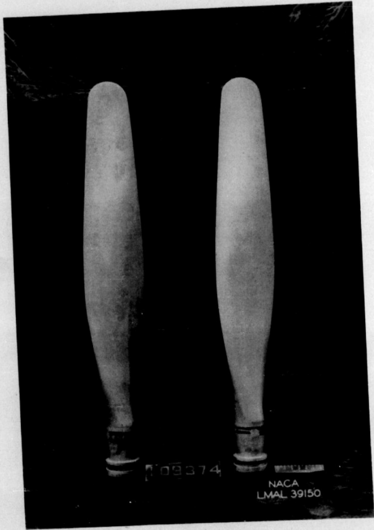
Figure 7.- Propeller blades 109374 (no trailing-edge extension) - cambered face (upper surface).
