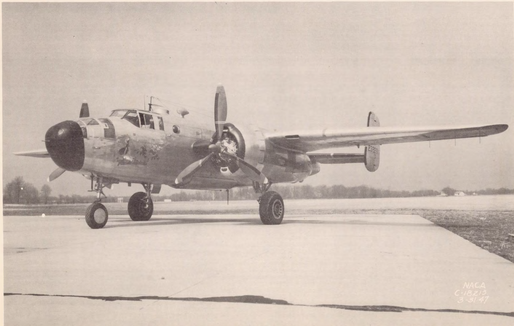
XB-25E WITH THERMAL ANTI-ICING EQUIPMENT FIGURE 1.
