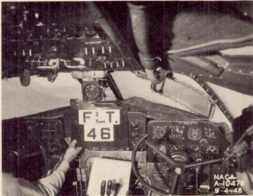
Figure 11.- Flush windshield of C-46 airplane showing ice protection afforded by the external heated-air jet, left side, and the electrically heated flush panel, right side.
