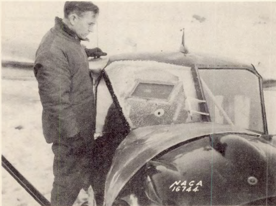
HEATED SECTION ON AIRPLANE WINDSHIELD FIGURE 11.
