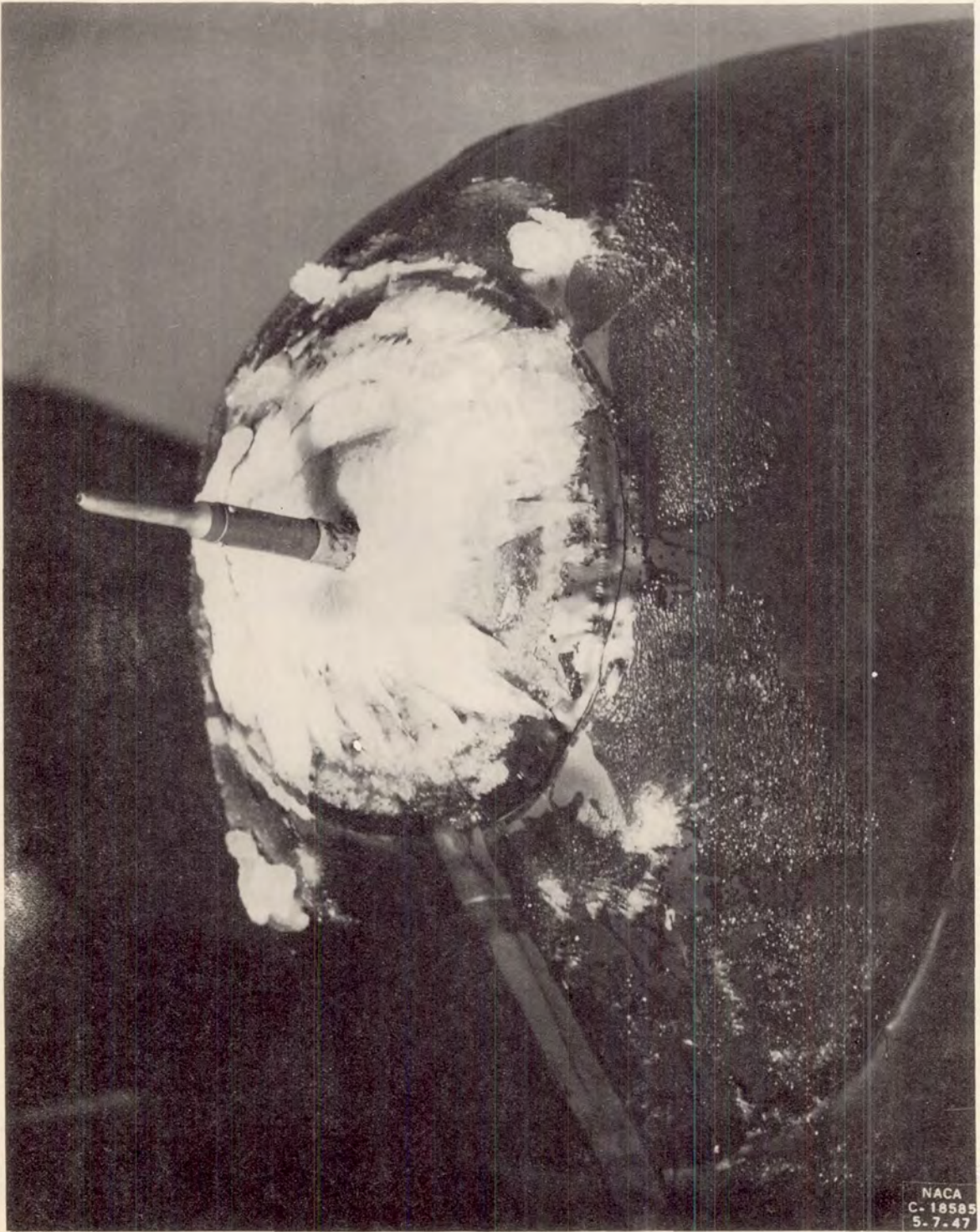
ICE ON NOSE OF FUSELAGE FIGURE 9.
