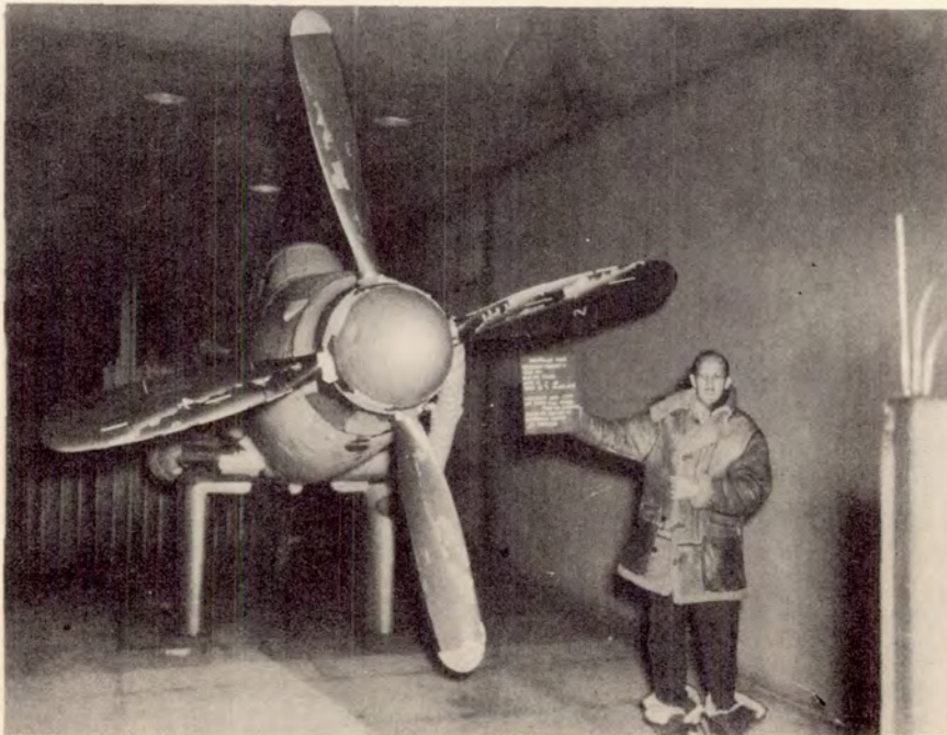
25% PARTITIONED BLADE RESIDUAL ICING FIGURE 15.
