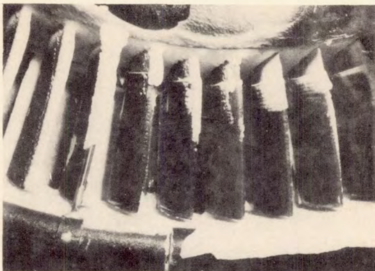
ICE ON HEATED FAN BLADES
