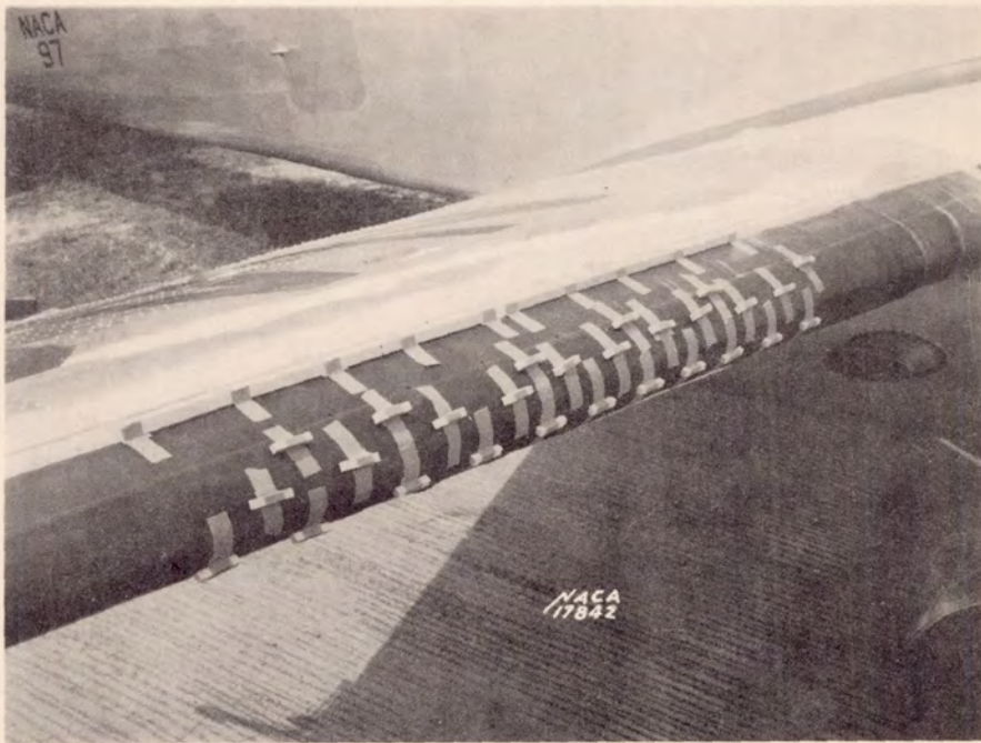
PROTUBERANCES ON WING LEADING EDGE SIMULATIONS OF ICE FIGURE 1.
