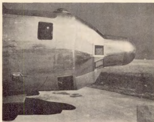
Figure 6.- General arrangement of windshield panels as tested on the B-24 airplane during the winter of 1946-47.
