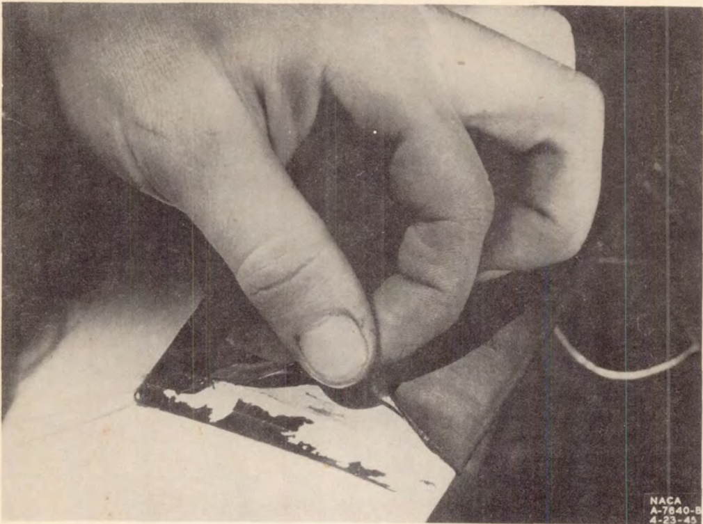
HAIL DAMAGE TO DE-ICING SHOE FIGURE 11.
