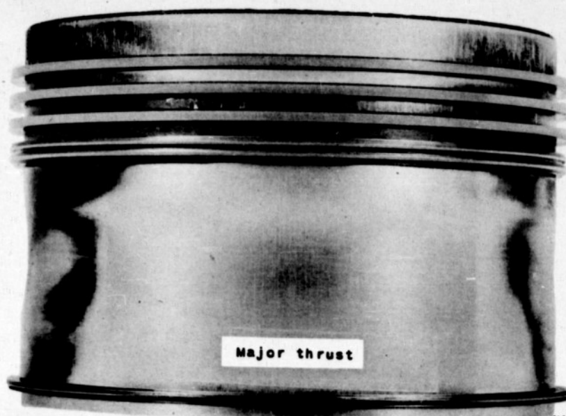
Figure 12. - Condition of major-thrust face of piston operated in previously used porous chrome-plated straight-bore cylinder barrel after test 7.
