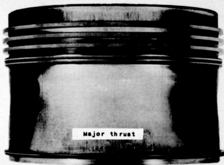
Figure 11. - Condition of major-thrust face of piston operated in straight-bore porous chrome-plated cylinder barrel after test 1.
