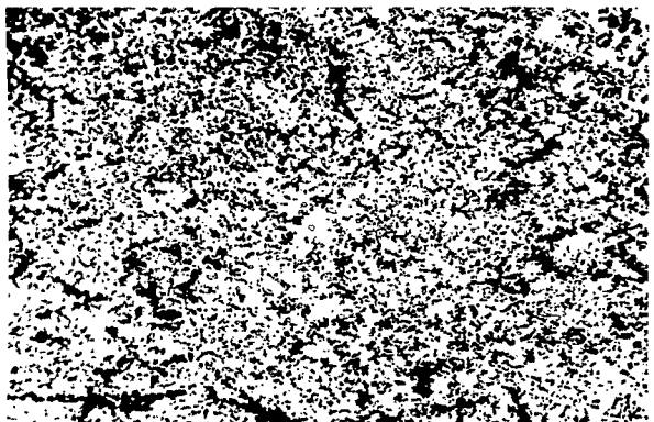
Figure 15.- Structure of the DVL-alloy, forged and precipitation hardened, X 100.
