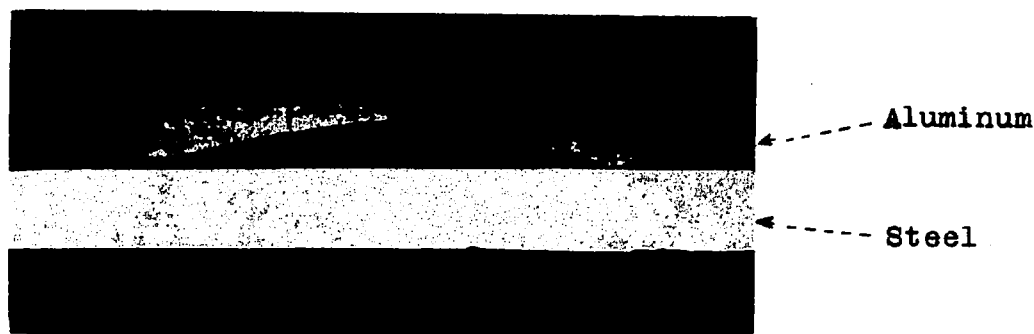
Figure 7.- Photomicrograph of aluminum welded to steel. Etched with 1.5 percent HF. Black area in aluminum sheet is the fused zone or weld nugget. 12 x
