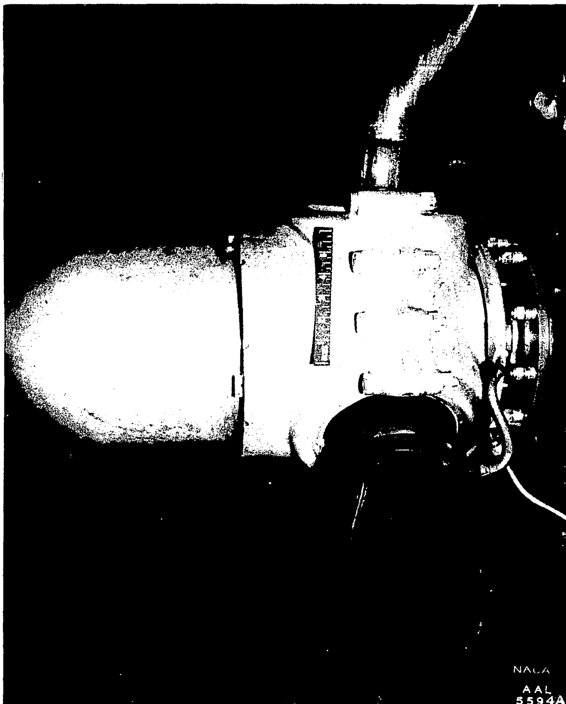
Figure 3.— The B. F. Goodrich Co. propeller alcohol feed rings installed on the propeller blades of the C-46 airplane.
