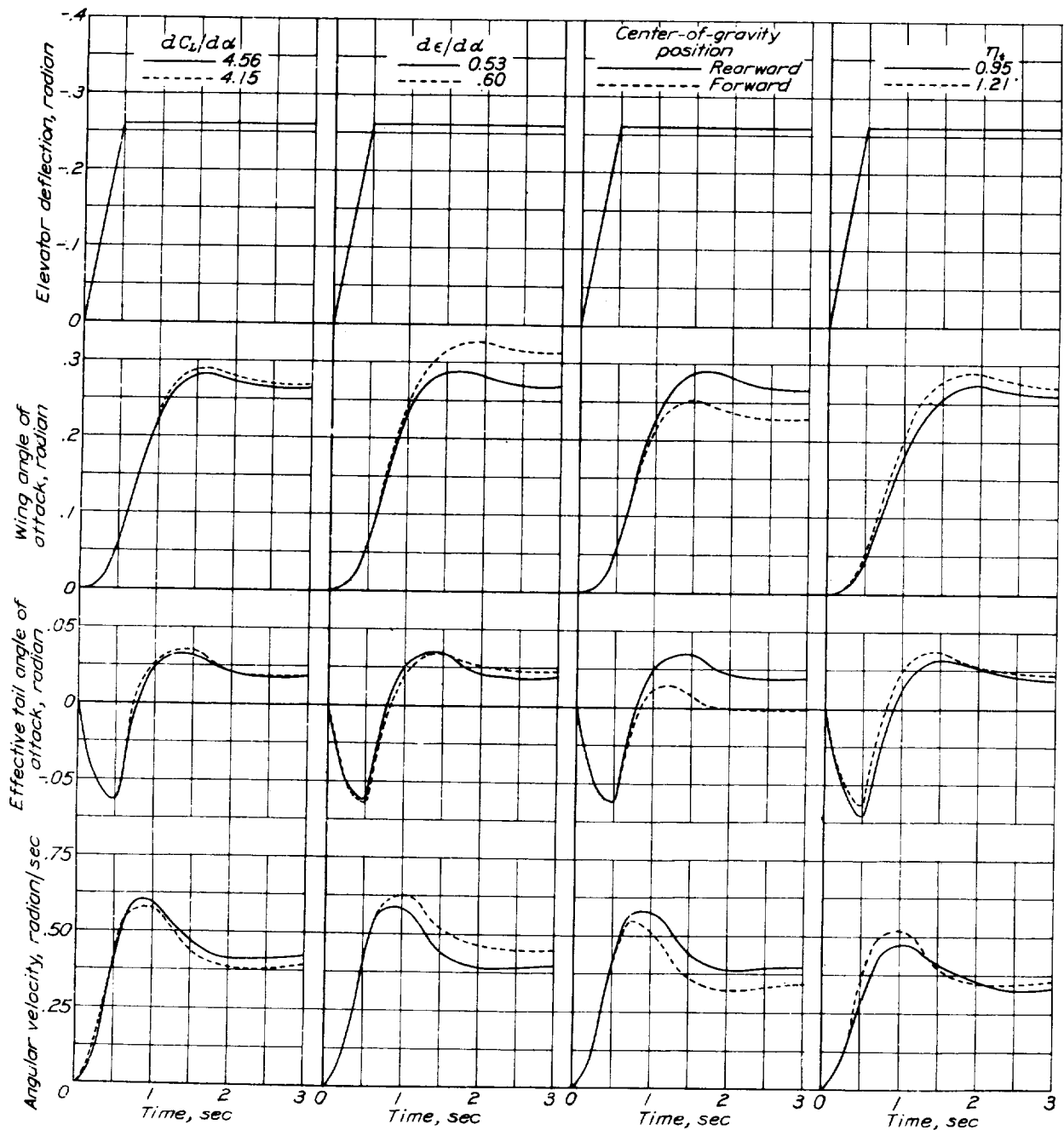
Figure 8.- Effect of downwash factor d\epsilon/d\alpha on increments of wing and tail angle of attack. Cases 4 and 9.
