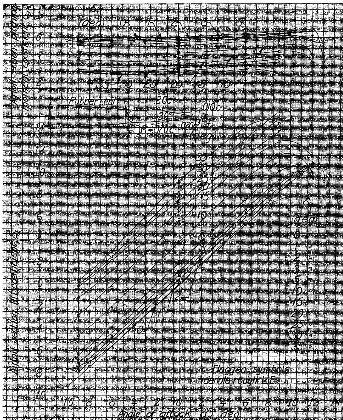
Figure 3.- Aerodynamic section characteristics of an NACA 0009 airfoil having 0.20c flap with 30° beveled trailing edge. Sealed gap, q = 15 pounds per square foot.
