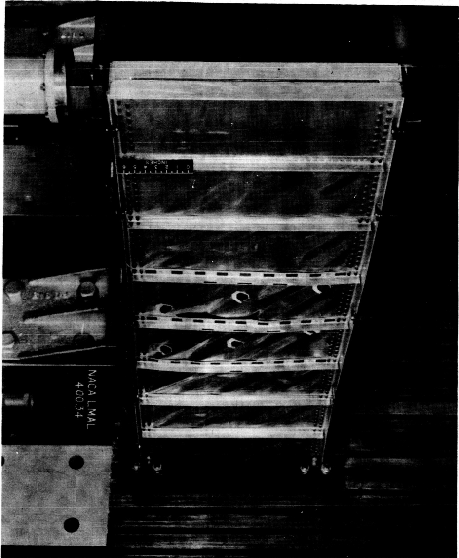
Figure 4.- A typical test beam after failure.
