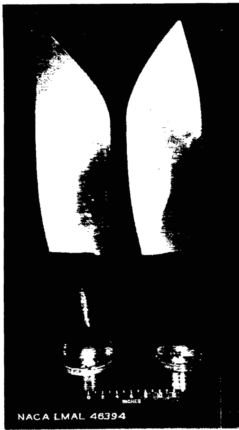
Figure 4.- Propeller blade with swept-back tip (left) and straight tip (right). Thrust surface.
