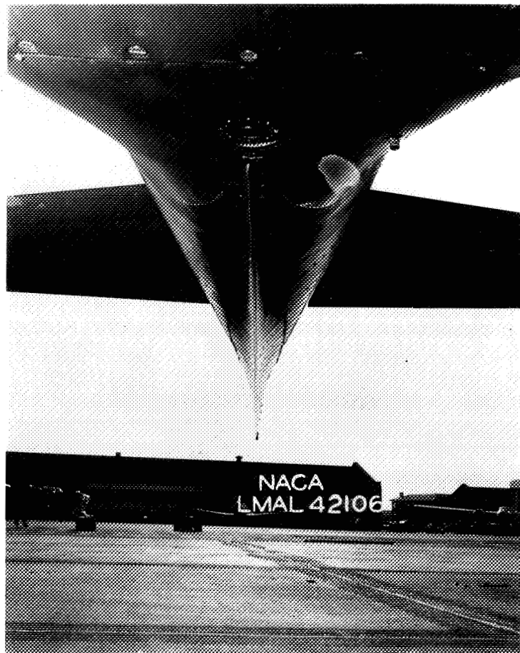
Figure 5.- Detail view of ventral fin showing sharp edge and cross-section.
