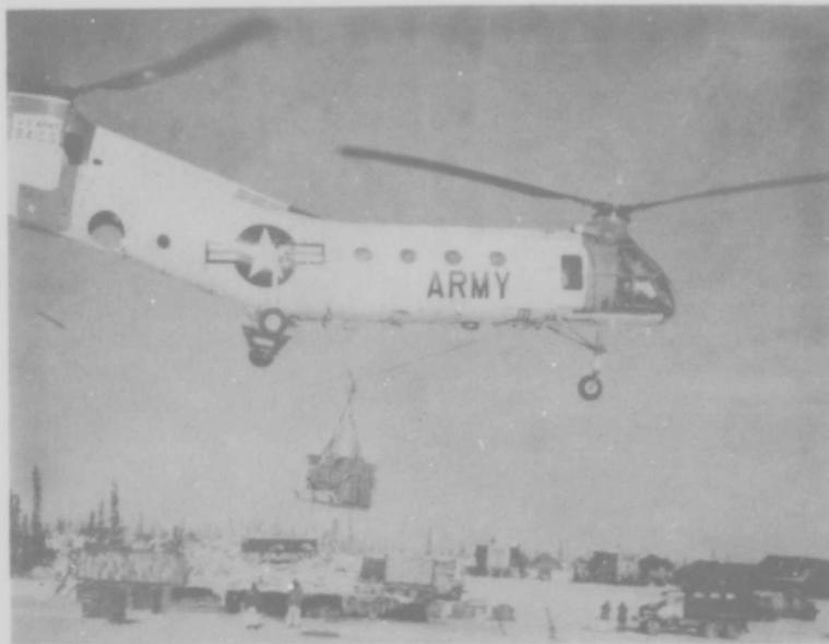
Figure 3 (Part V) to Section V. Utilization of externally rigged sled pallet for H-21 Helicopter delivery of supplies to forward platoon emplacements of US Forces.
