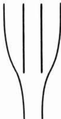
ATOMIC MODEL OF EDGE DISLOCATION IN GRAPHITE (3)
