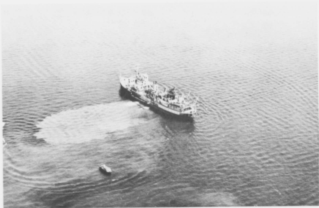
Photo 10 Washing Out Hopper Bins at Disposal Site
