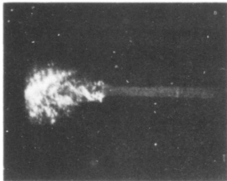
Figure 3A. Beginning of cycle. The gases have reached their maximum exhaust velocity at the tailpipe exit (left side) and the pressure is falling in the combustion chamber.
