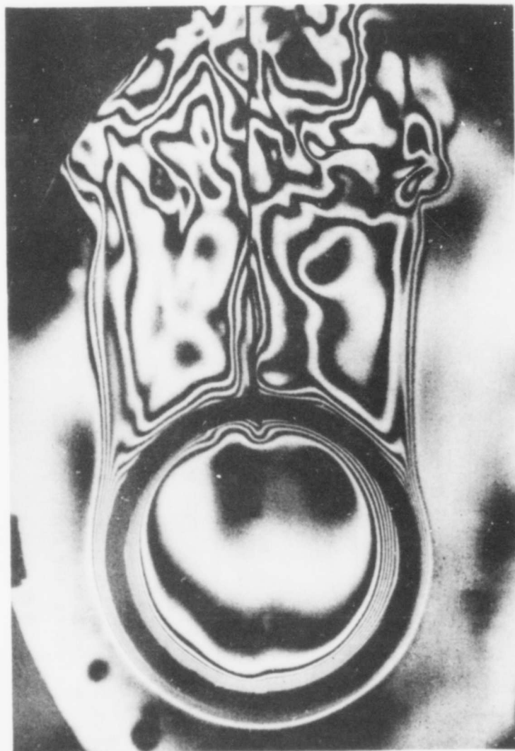
Figure 8 Interferometric photograph of heated air rising from a heated metal ring (axial length 1/2 ", diameter 4-1/2 ", wall thickness 1/4 ") taken with system shown in Figure 9.
