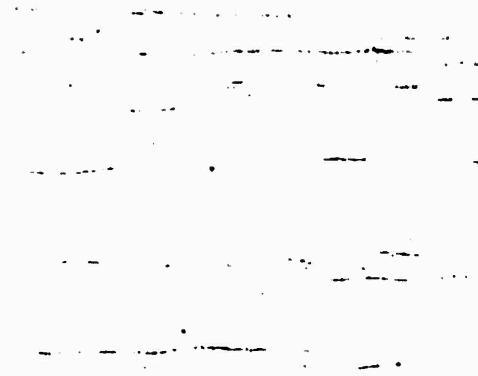
X100 -B- Unetched Poor quality steel. Very high concentration of elongated inclusions.
