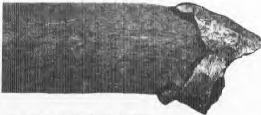
.40 C REPUBLIC ARMOR -45^{\circ} DV BEVEL GEOMETRY IMPROVED WITH LARGER ANNEALING BEADS.
