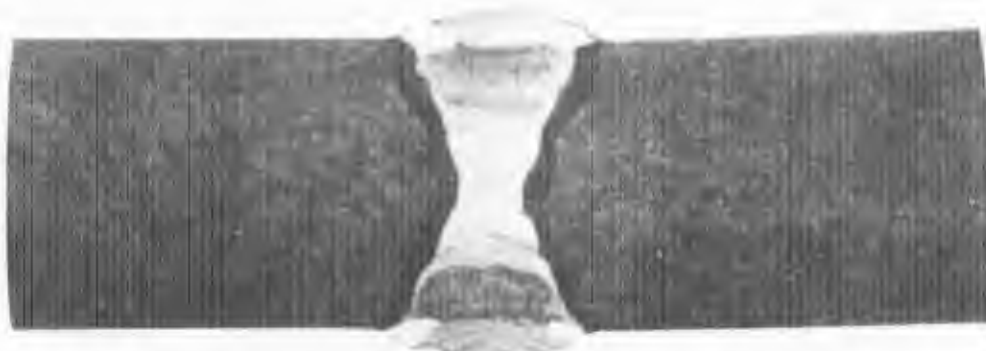
Macroetched transverse section through undamaged portion of weld joint.
