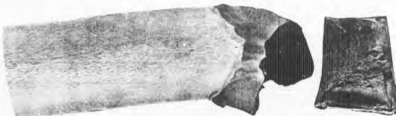
Bend bar fracture.
