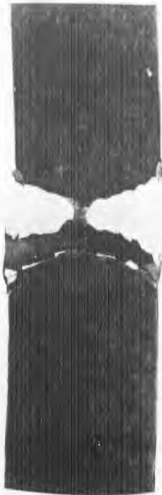
Macroetched transverse section through ballistic fracture.
