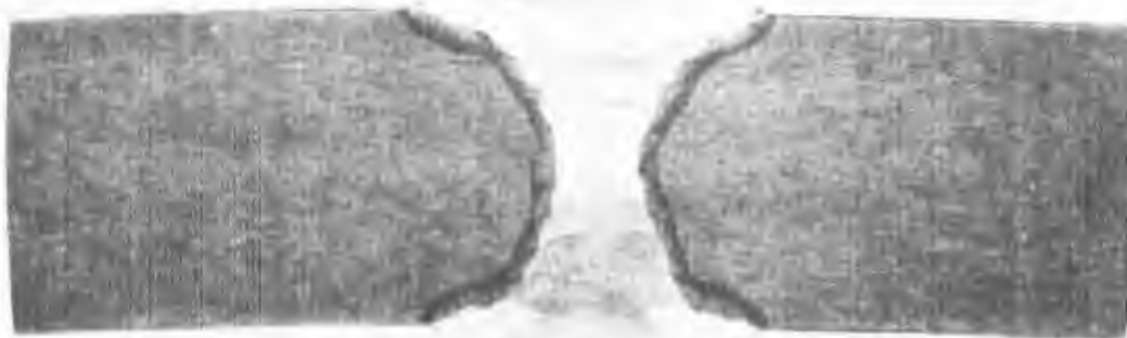
Macroetched transverse section through undamaged portion of weld joint.
