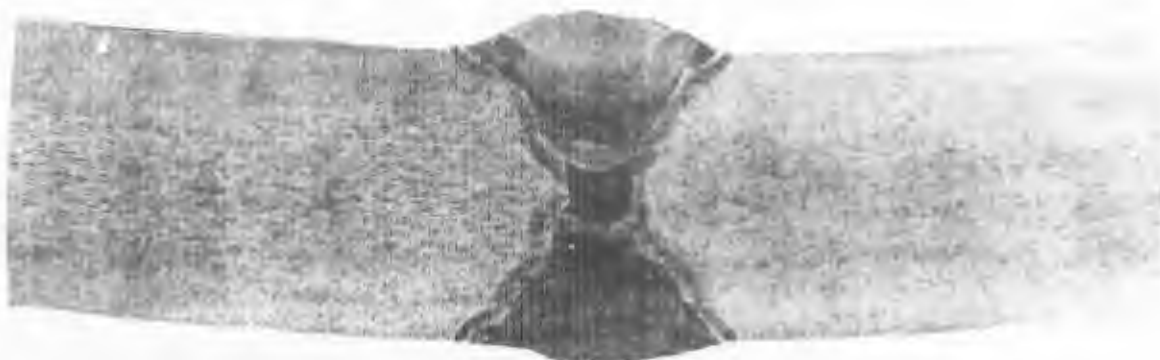
Macroetched transverse section through undamaged portion of weld joint.
