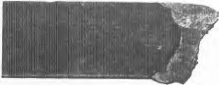
.26 C JONES AND LAUGHLIN ARMOR -45^{\circ} DV BEVEL - GEOMETRY IMPROVED WITH LARGER ANNEALING BEADS.
