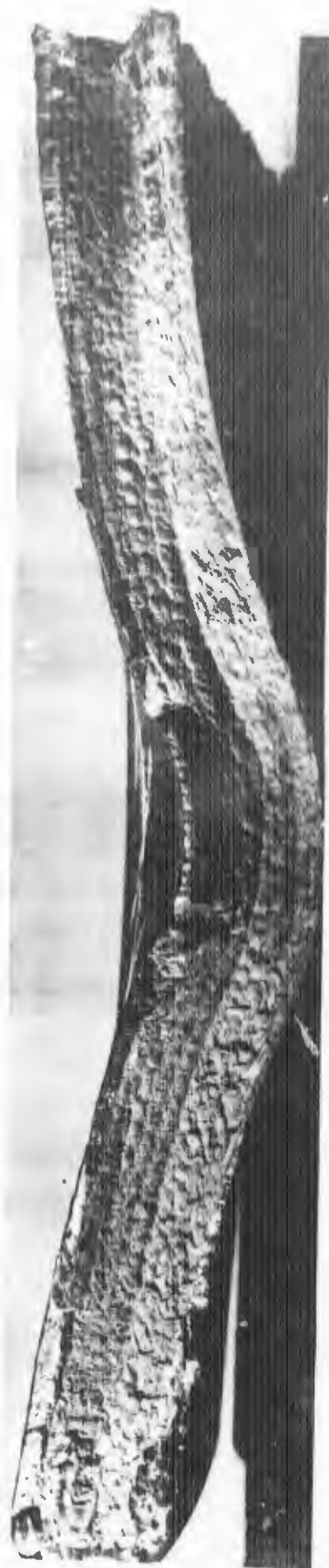
Ballistic fracture surface, weld metal side.
