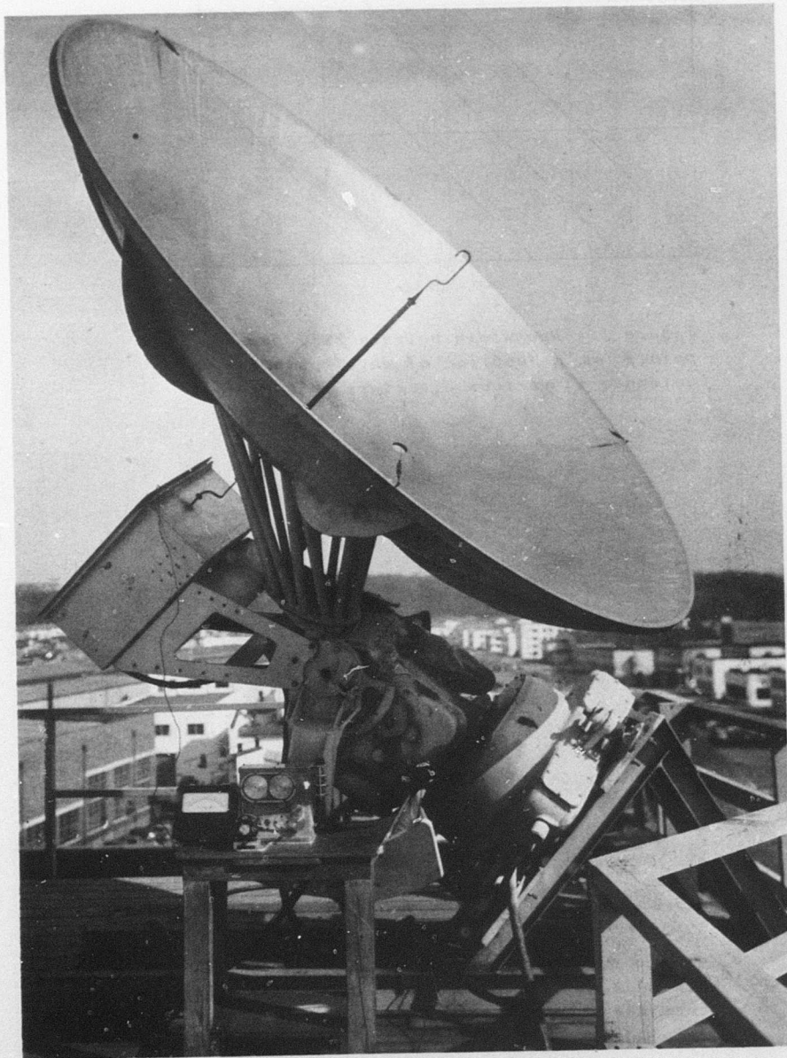
Figure 3 - Ten-foot diameter parabolic antenna with 8.5-millimeter feed horn
