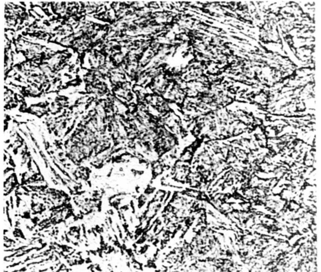
X1000 MA-4250 Nital and Picral Etch
