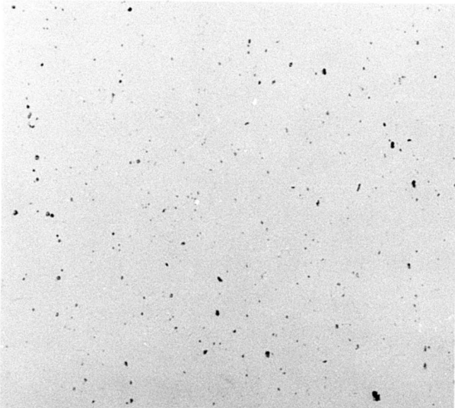
X25 MA-4207 Unetched. Distribution of nonmetallic inclusions. Relatively clean steel.
