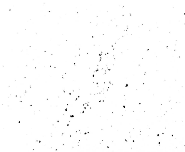
X25 MA-4155 Unetched. Distribution of nonmetallic inclusions.
