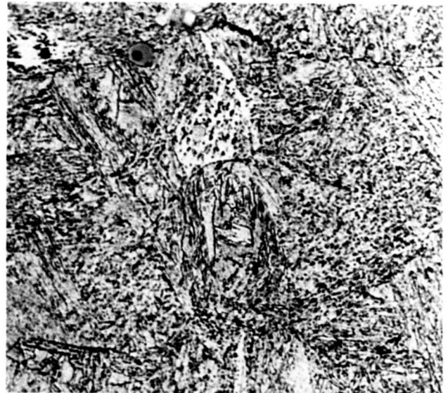
MA-4254 X1000 Nital and Picral Etch MA-4254
