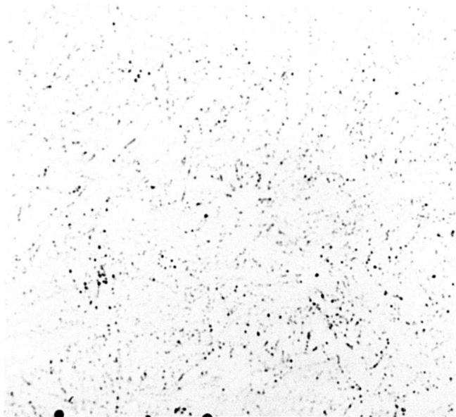
X1000 MA-4191 Murakami Etch - Random carbide distribution.
