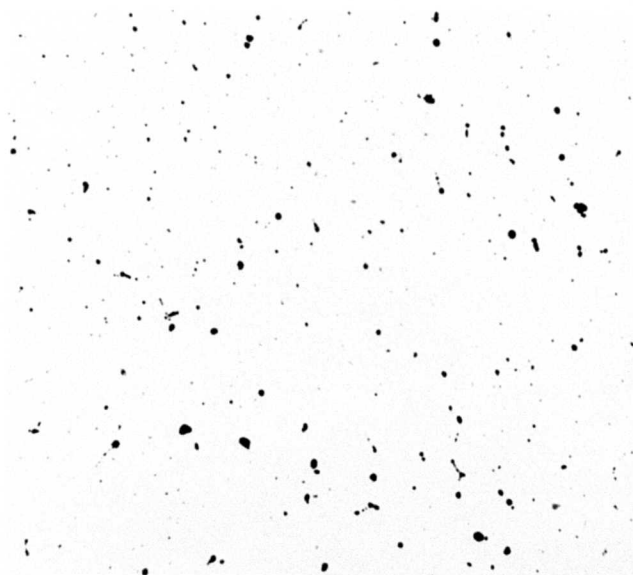
X25 MA-4256 Unetched. Distribution of nonmetallic inclusions.
