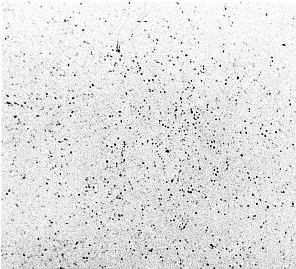
X1000 MA-4183 Murakami etch. Random distribution of carbides.
