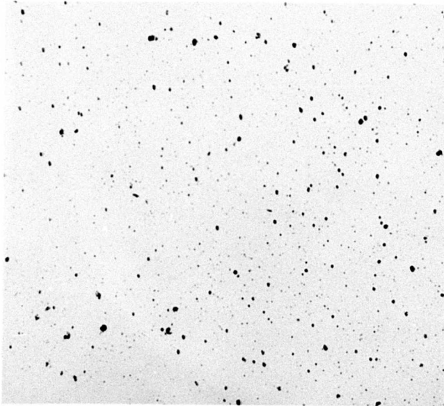
X25 MA-4206 Unetched. Distribution of nonmetallic inclusions.
