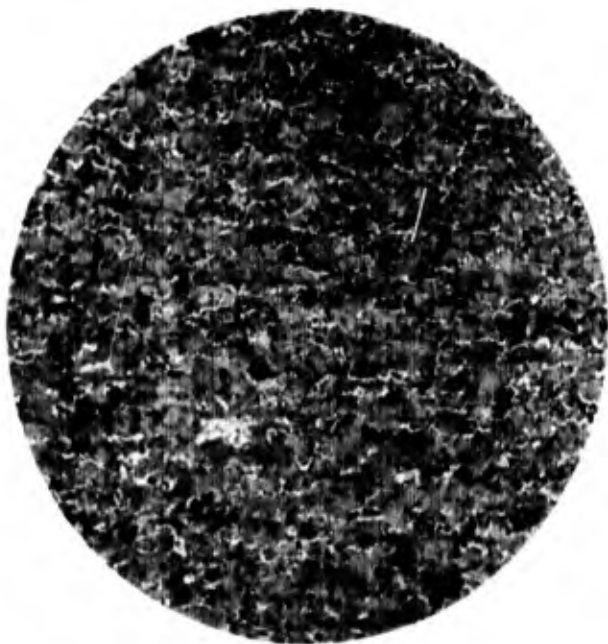
Figure 103. Heat No. 7345. Microstructure of the as-rolled 3/4-in. plate. X100
