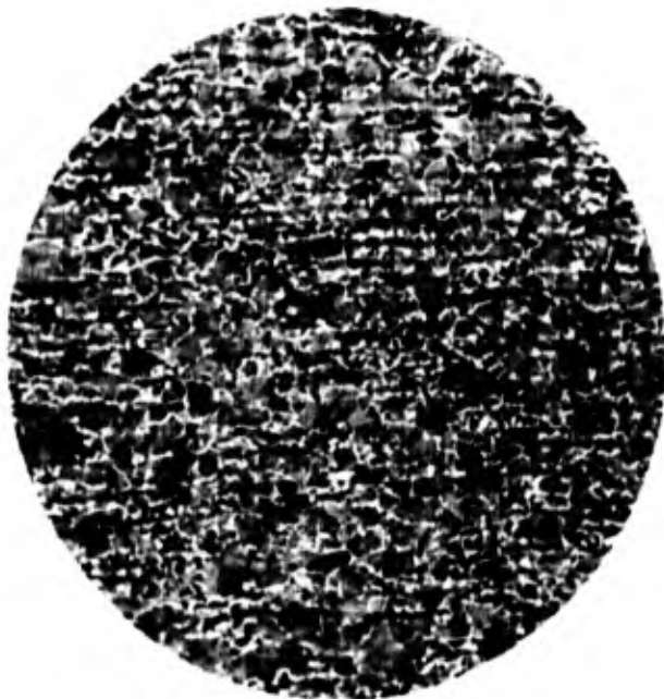
Figure 109. Heat No. 7352. Microstructure of the as-rolled 3/4-in. plate. 13333 X100
