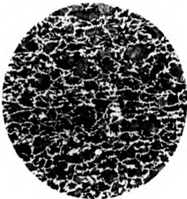
Figure 93. Heat No. 7326. Microstructure of the as-rolled 3/4-in. plate. X100
