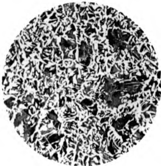
Figure 87. Heat No. 7277 - Repeat on Heat 7091 (Aluminum treated). Microstructure of the as-rolled 3/4-in. plate. 13311 X100
