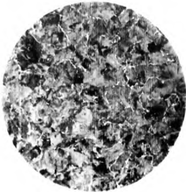
Figure 86. Heat No. 7276 - Repeat on Heat 7092. Microstructure of the as-rolled 3/4-in. plate. 13310 X100
