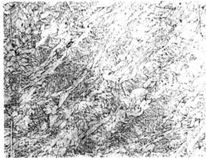
Fig. 11 10% Nital x100 Weld structure - position #2
