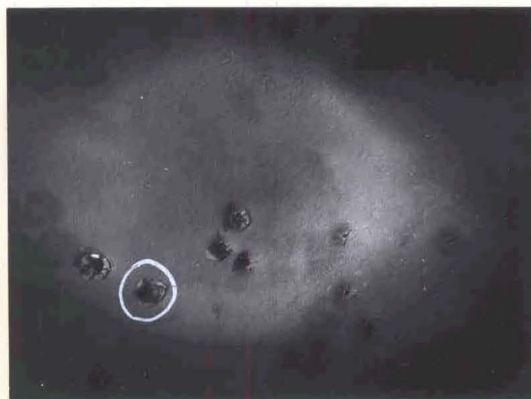
Figure 18 - Back face of plate. Fragments blown off. Photographs taken by reflected light. Ammunition Caliber .30 Armor Piercing service velocity at a distance of 100 yards.
