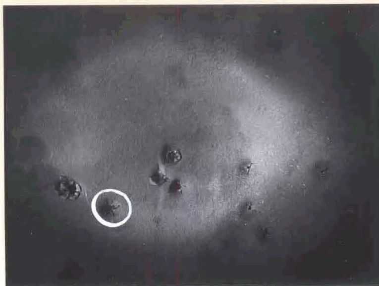
Figure 17 - Back face during impact. Nose of bullet core appearing through back of plate.
