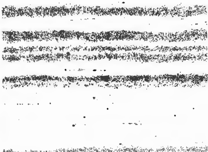
Sample No. RH 11792 - 1 1/2" thick. Pronounced banding associated with sulphide-oxide-silicate inclusions. "Woody" fracture. Failed PTP test.
