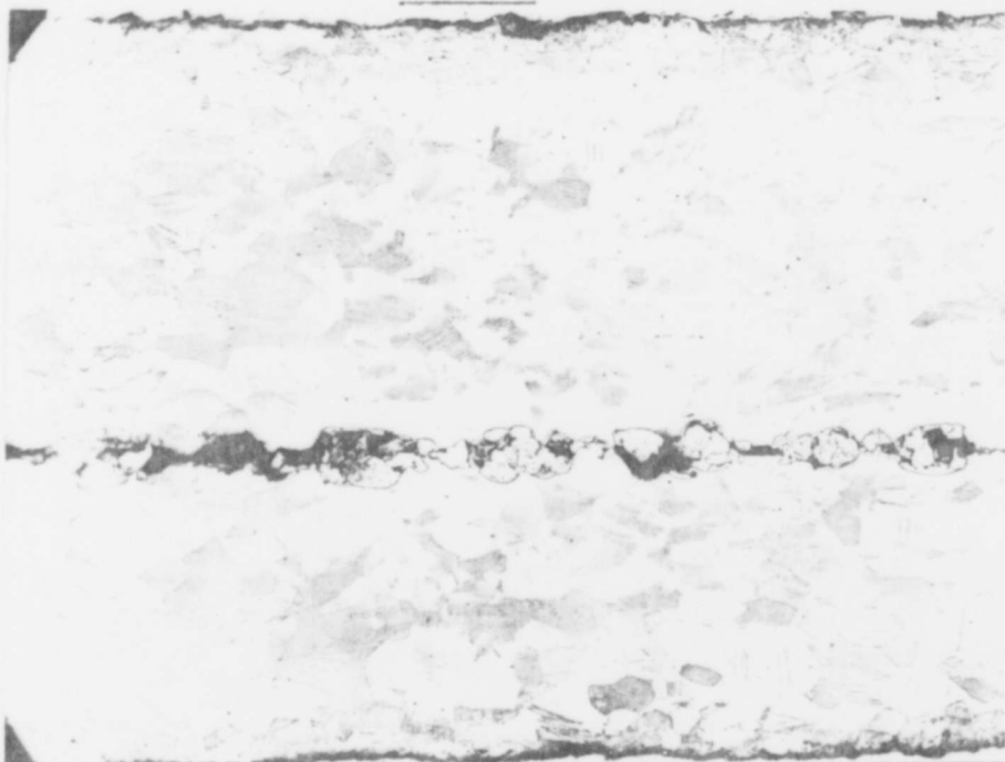
Nital Etch -A- X100 Steel D. Streak of martensite into which crack resulting from deep drawing extends.
