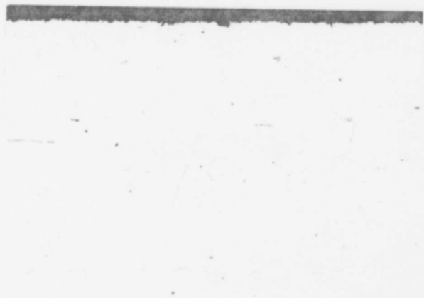
Steel E. -A- X100 Satisfactory for helmet application. No decarburization.
