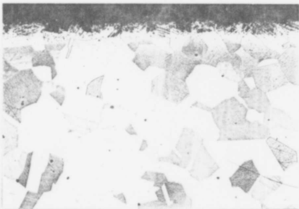
-E- X100 Sharon "Rough Surface". Decarburized surface typical of Sharon and Carnegie STEEL PRODUCED AT GOVERNMENT EXPENSE
