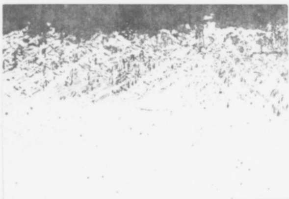
-F- X750 Sharon "Rough Surface". Martensite level surface. 0.0017" layer de- carburized to martensite. 12
