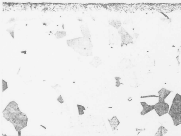
Nital Etch -A- X100 Steel A. Surface decarburization. 0.0025" thick layer of martensite.
