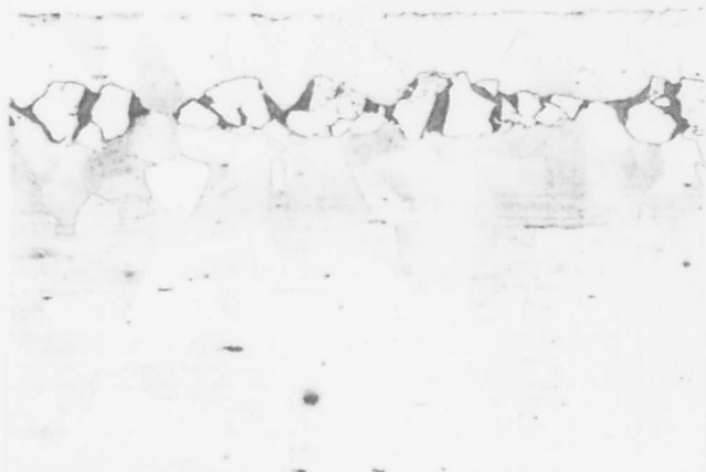
Nital Etch -C- X100 Steel C. Streak of fragmented grains of martensite, probably residual ingot piping rolled out in sheet.
