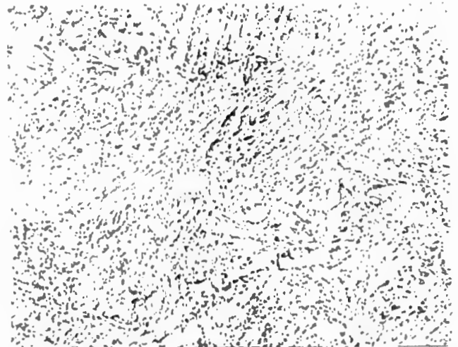
Pical steel Incompletely quenched structure. Martensite tempered pearlite and
