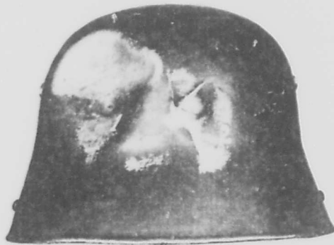
GERMAN HELMET AFTER BALLISTIC TEST MARCH 20 1942 W.A.710-1792-C
