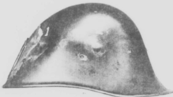
DUTCH HELMET AFTER BALLISTIC TEST MARCH 20 1942 W.A. 710-1790-C
