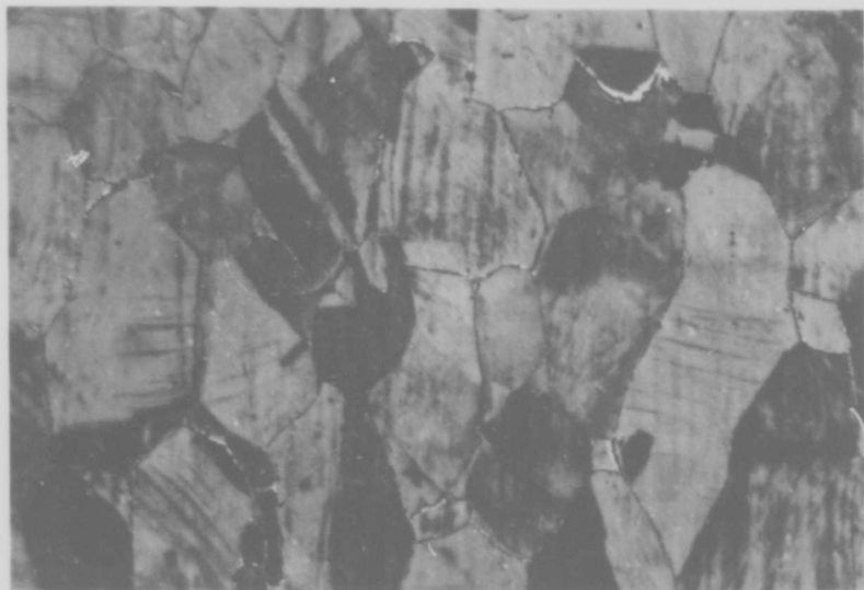
FIGURE 4 HELMET SHEET QUENCHED FROM 1475°F AND REDUCED 16% BY COLD ROLLING X 250
