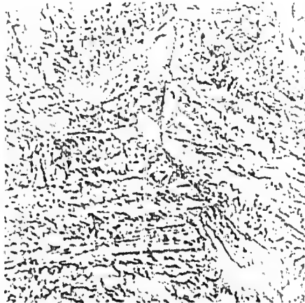
FMP-11 -c- X1000 Ferrite and high temperature transformation products.
