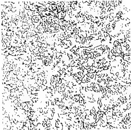
-c- X1000 Microstructure of strip G. Martensite and ferrite. Hardness - 375 VPN.
