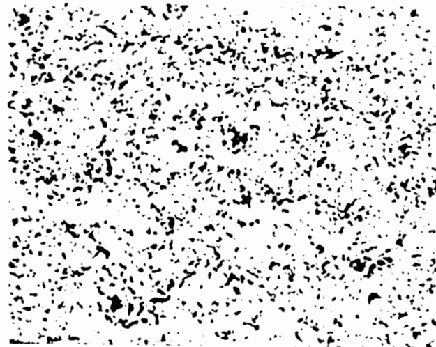
No. 4776-2-1. Fairly uniform sorbite and possible traces of ferrite. Typical of plates 4776-15-3, 19296-2-1A, 19296-1, and 19296-3.
