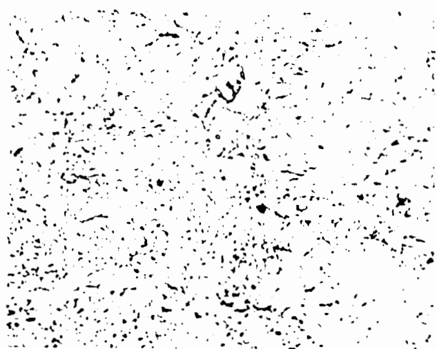
X1000 R45 Picral Tempered martensite and occasional grain boundary ferrite. BHN 373.
