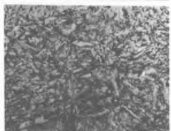
X1000 F Picral Plate 4 - Tempered martensite.
