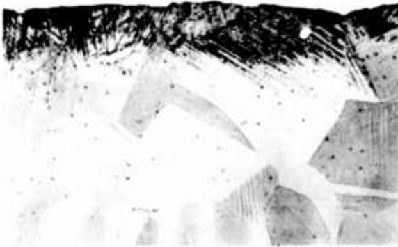
-A- X250 Helmet D4, McCord Lot 544B, Carnegie Heat 255739. Martensitic surface layer resulting from decarburization. Width of layer - 0.0016". Magnetic Traverse - 23.0".
