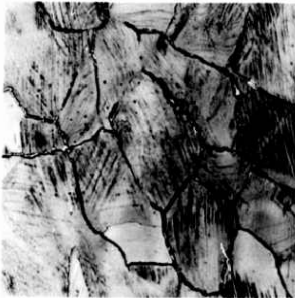
-C- X1000 Helmet E1, McCord Lot 541C, Sharon Heat 72203. Network of undissolved carbides at grain boundaries. Magnetic Traverse - 3.0".
