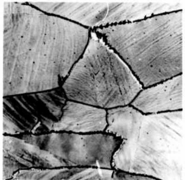
-D- X1000 Helmet E2, McCord Lot 549B, Sharon Heat 72198. Undissolved carbides. Magnetic Traverse - 1.0".
