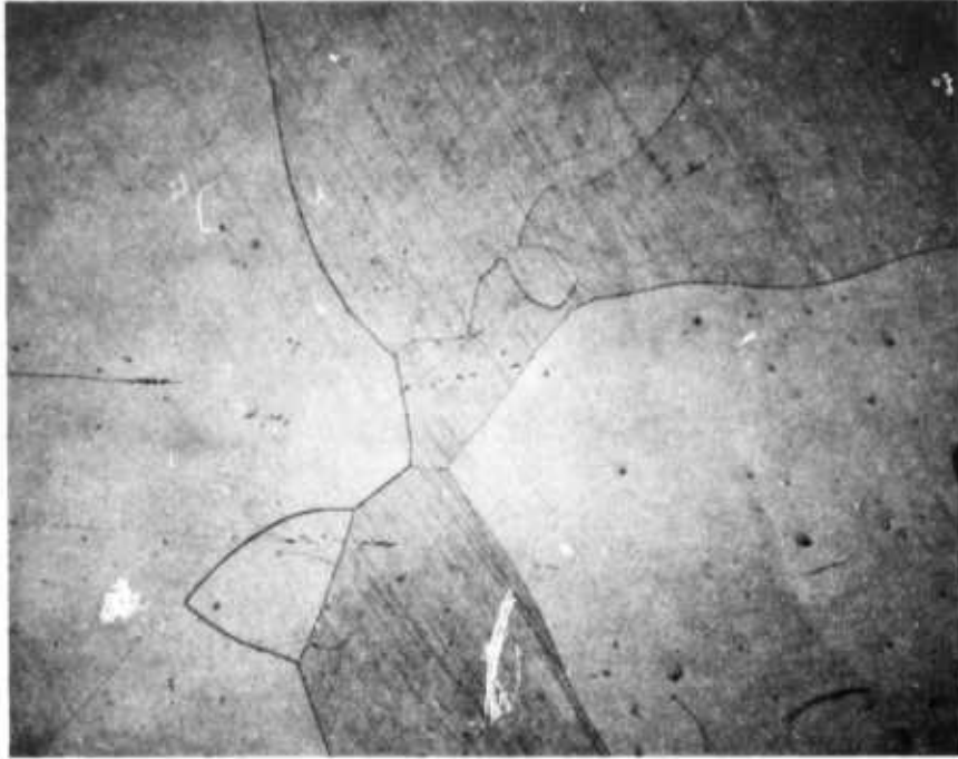
Fig. 6-13 Photomicrograph of VHP-154. Hot Forged \text{CaF}_2 at 1000^\circ\text{C} 79 percent reduction in thickness. 25X
