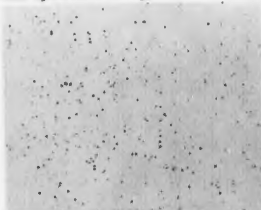
Heat No. 12. Specimen No. 12A5 Austenitized 4 hours at 1550°F. Many undissolved carbides.
