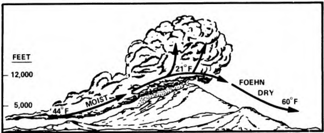
Figure 2-17 The Chinook or Föhn wind. (From Kuenen, P. H., Realms of Water , Copyright © 1955 by John Wiley and Sons.)
