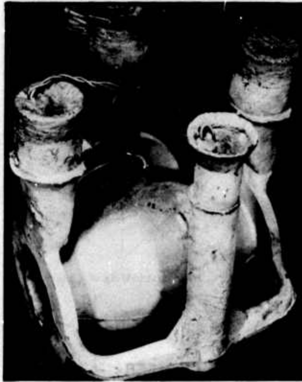
Figure 232. Globe valve - improved risering practice.
