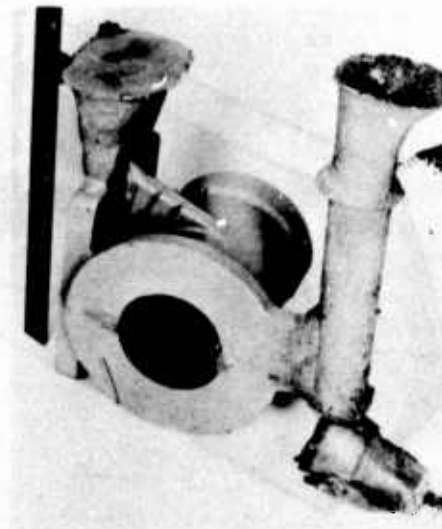
Figure 138. Cold metal riser. (Not Recommended)
