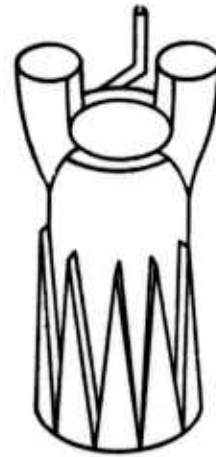
Figure 237. Tapered chills on a G metal bushing.
