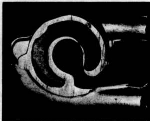
Figure 216. Misrun. (Caused by a core shift)
