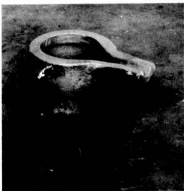
Figure 168. Crucible for tilting crucible furnace.
