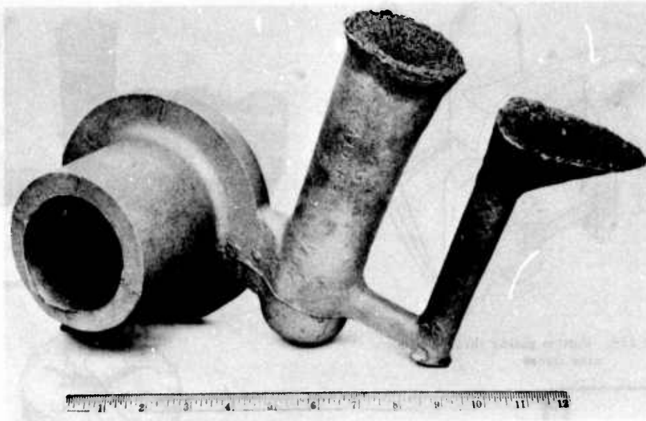
Figure 125. Parting gate through the riser.
