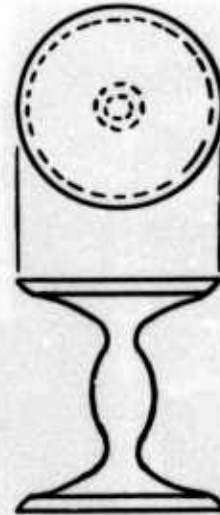
Figure 76. Recommended chaplet design for emergency use.
