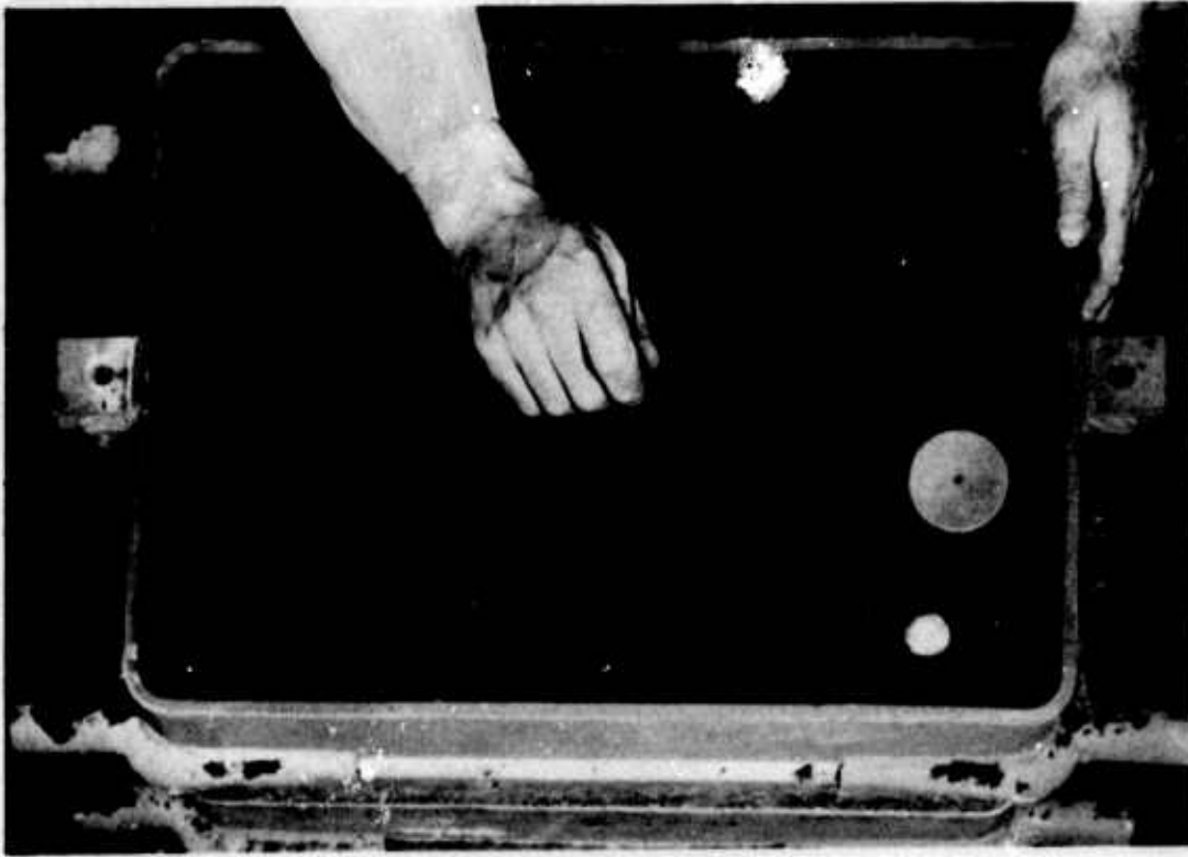
Figure 85. Venting the cope.
