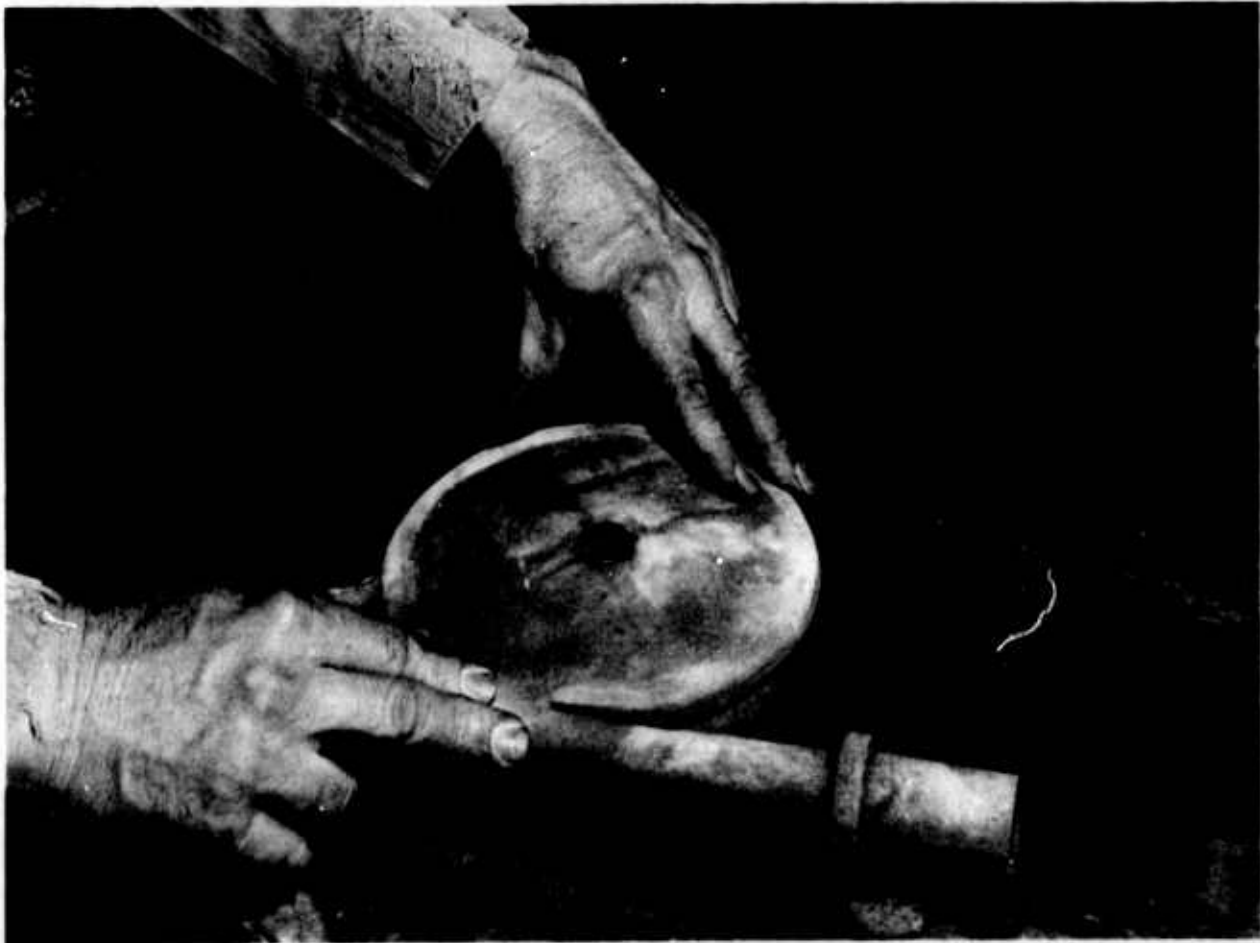
Figure 110. Assembling the two core halves.
