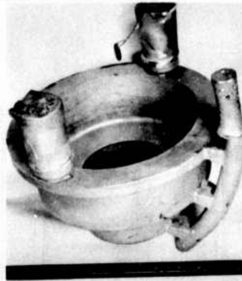
Figure 136. Proper riser size and shape.
