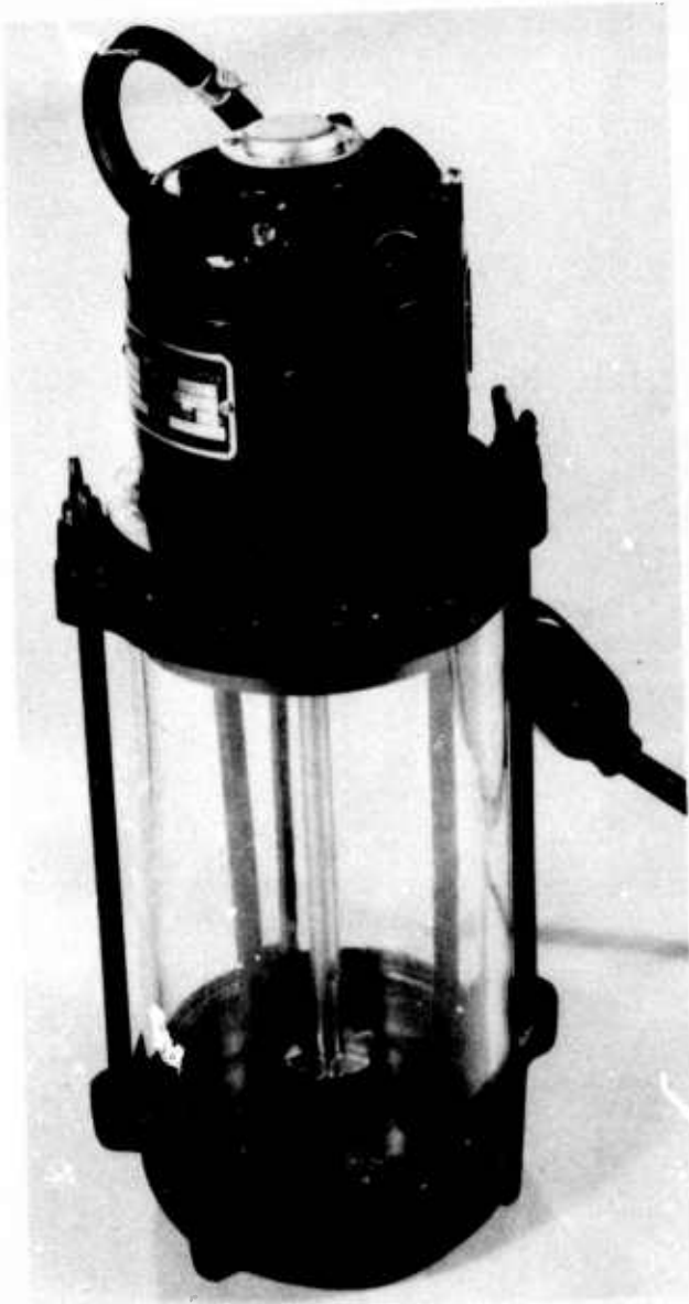
Figure 69. Sand washing equipment assembled.
