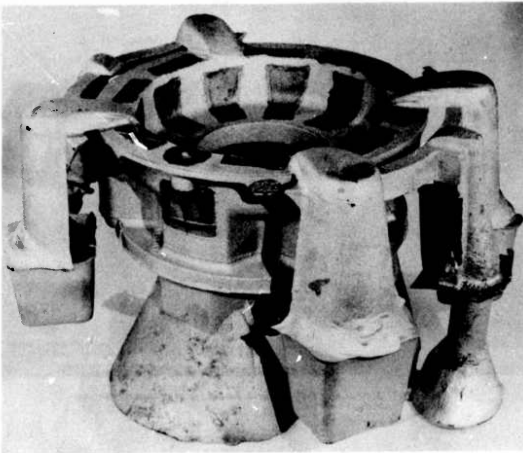
Figure 161. As-cast aluminum casting showing location of external chills.
