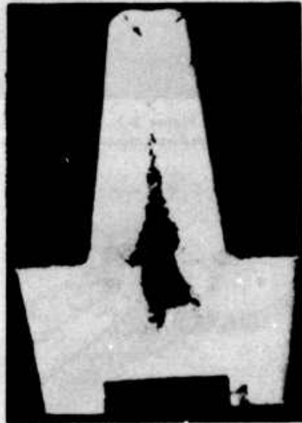
Figure 199. Gross shrink. (Caused by inadequate feeding)
