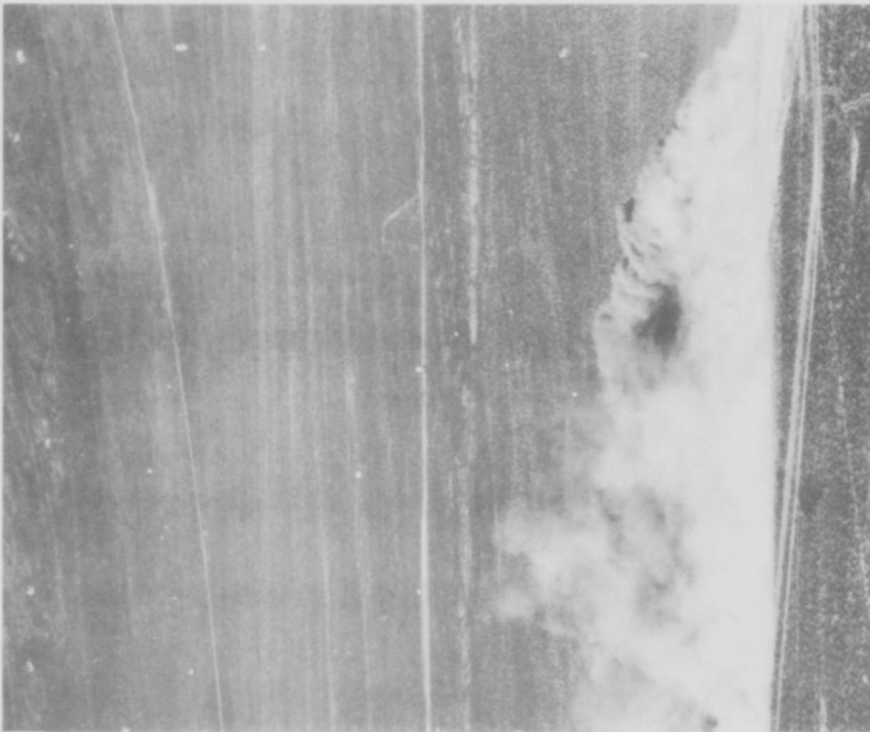
Fig. 3.11 HE-3. Time plus 40 seconds. 100 per cent base surge formation moving with wind toward left side of picture.
