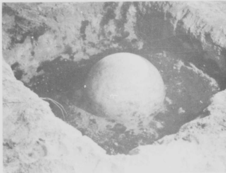
Fig. 3.2 177 Pound Pentolite Sphere
