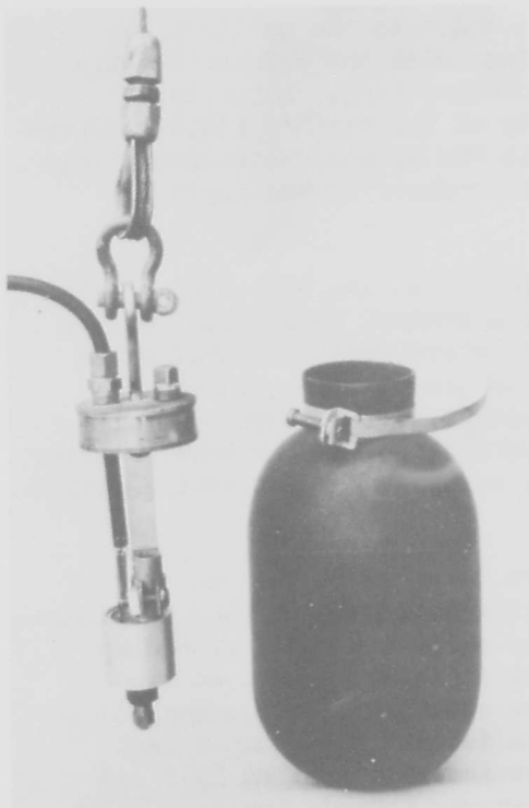
Fig. 3.5 Earth-Pressure Gage, Shown with the Neoprene Oil Bag
