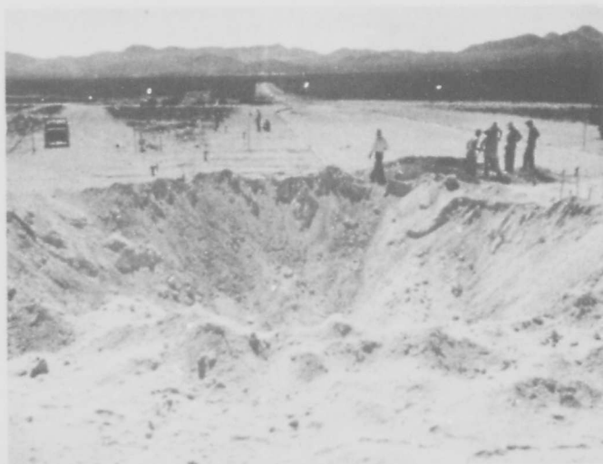
Fig. 4.2 Crater from Shot HE-2. The Underground Shot will probably be very similar with the diameter increased 3 \frac{1}{3} times.
