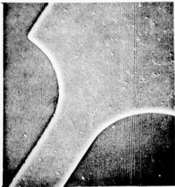
a) AFTER PHOTO-RESIST PROCEDURE 1000X SEM
