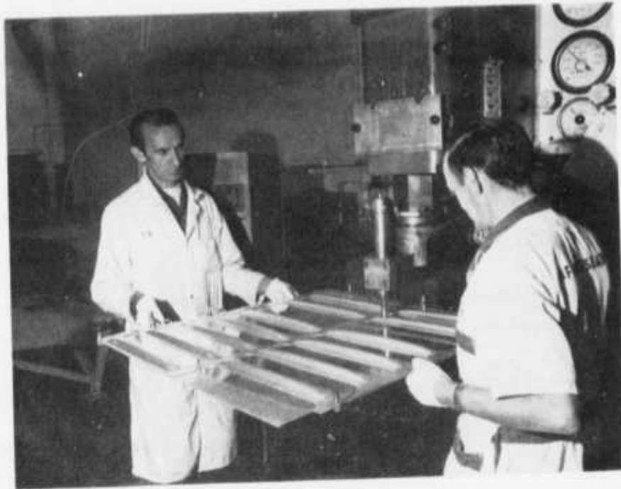
FIGURE 103 — TYPICAL SECTION OF THE C-130 TRAILING EDGE BEING JOINED BY WELDBONDING
