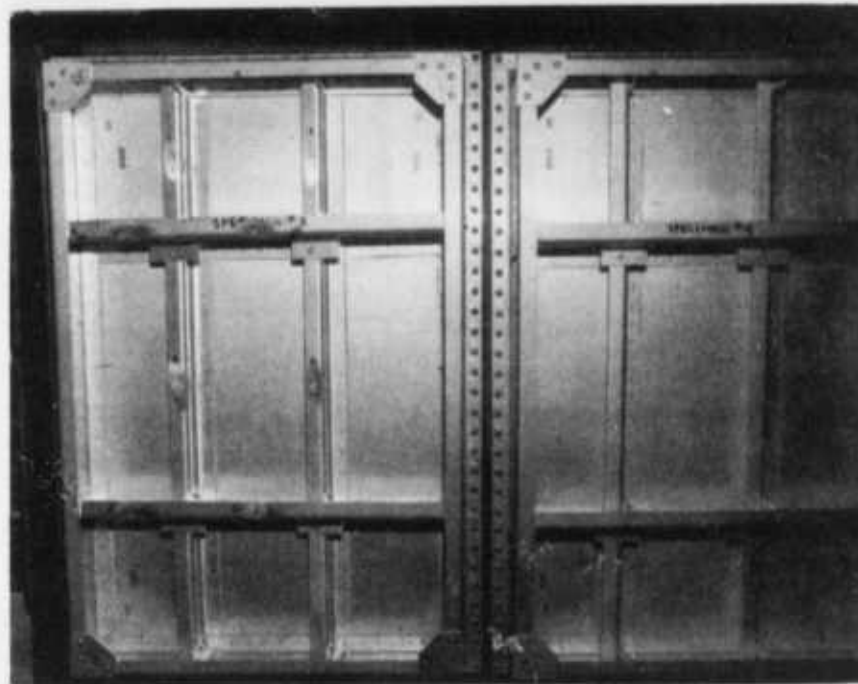
FIGURE 54 — FLAT WELDBONDED SUB-SCALE SONIC FATIGUE COMPONENTS INSTALLED IN ACOUSTIC FACILITY
