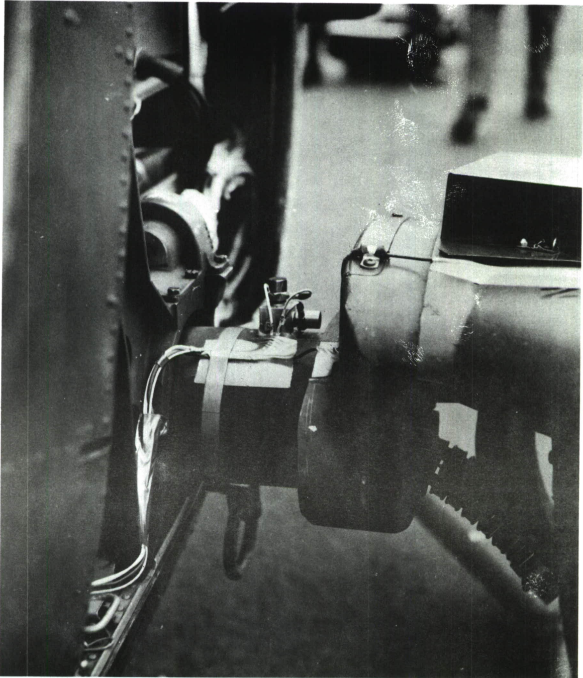
Figure 17. Piezoelectric Accelerometers, XM-27 Armament Mount, Sta. 92, PUID's 53, 54, 55
