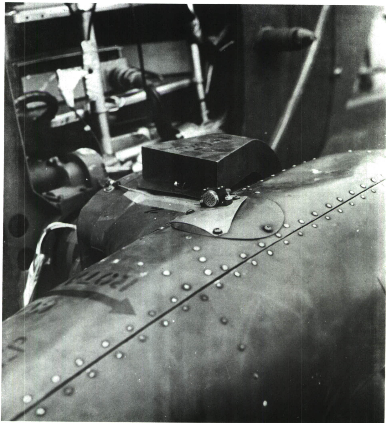
Figure 31. Microphone, XM-27 Armament Gun Pod, Sta. 90, PUID 69
