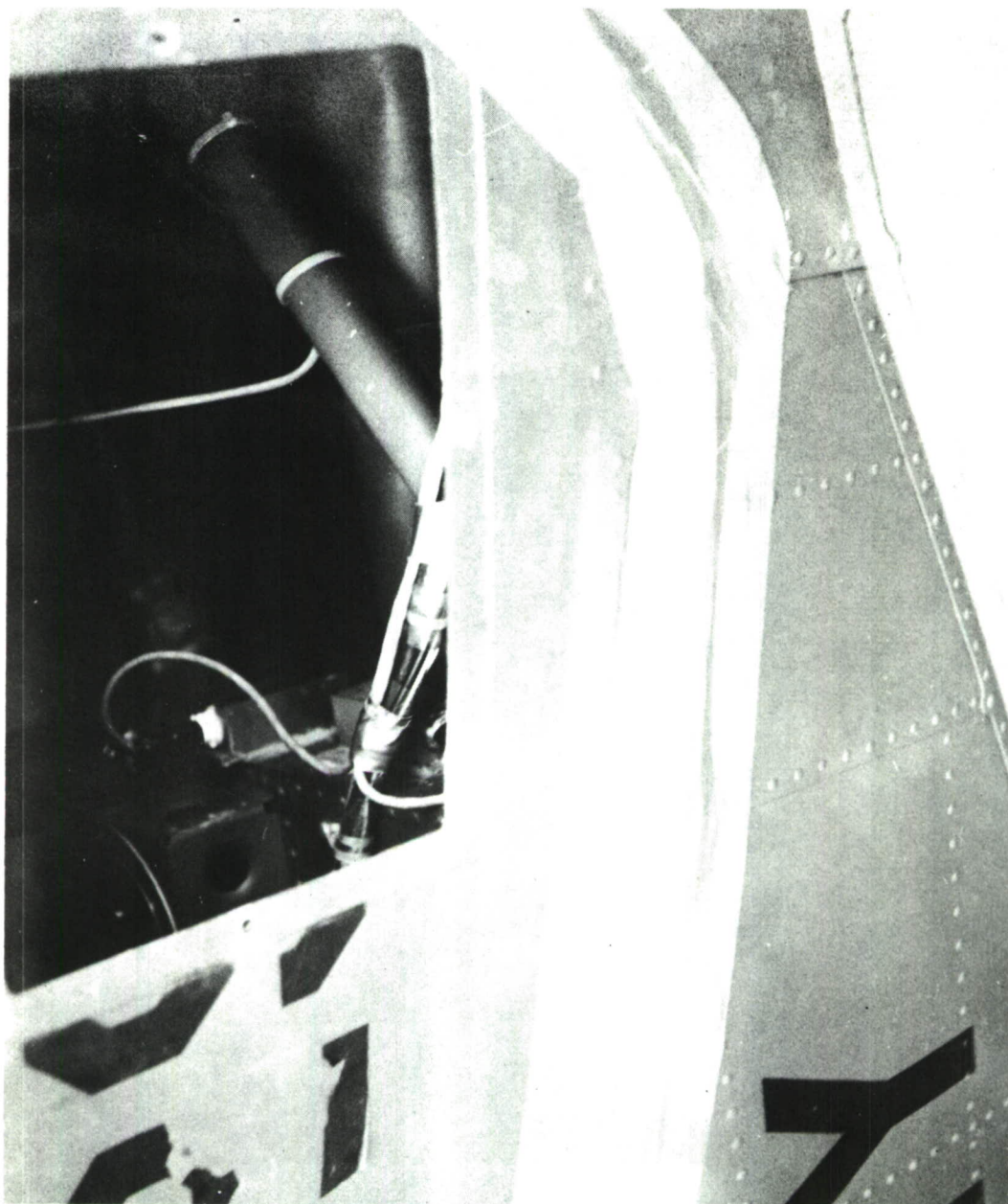
Figure 23. Low Frequency Accelerometers, Fuselage-Tail Section Interface, Sta. 130, PUID's 51, 63
