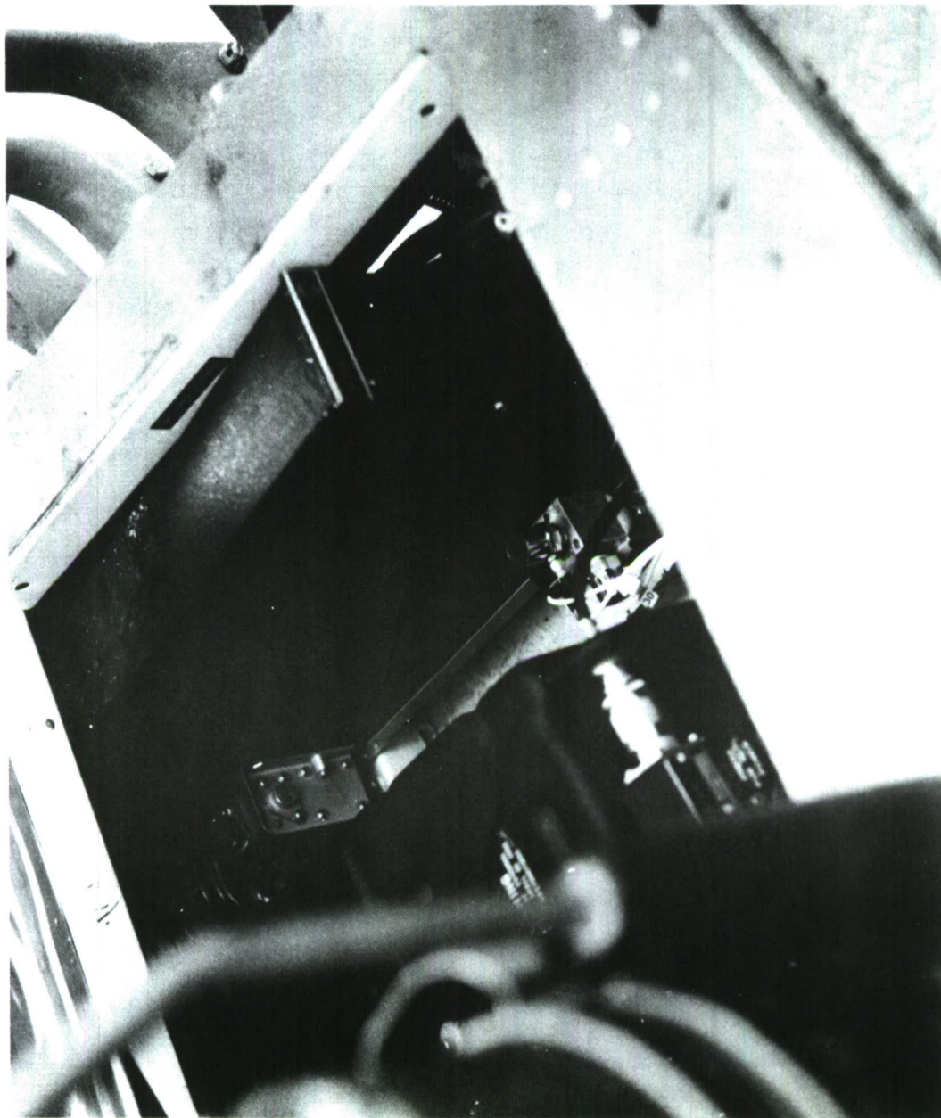
Figure 14. Piezoelectric Accelerometers, Electronic Compartment, Right Side, AN/ARC-51 Sta. 55, PUID's 32, 33, 34
