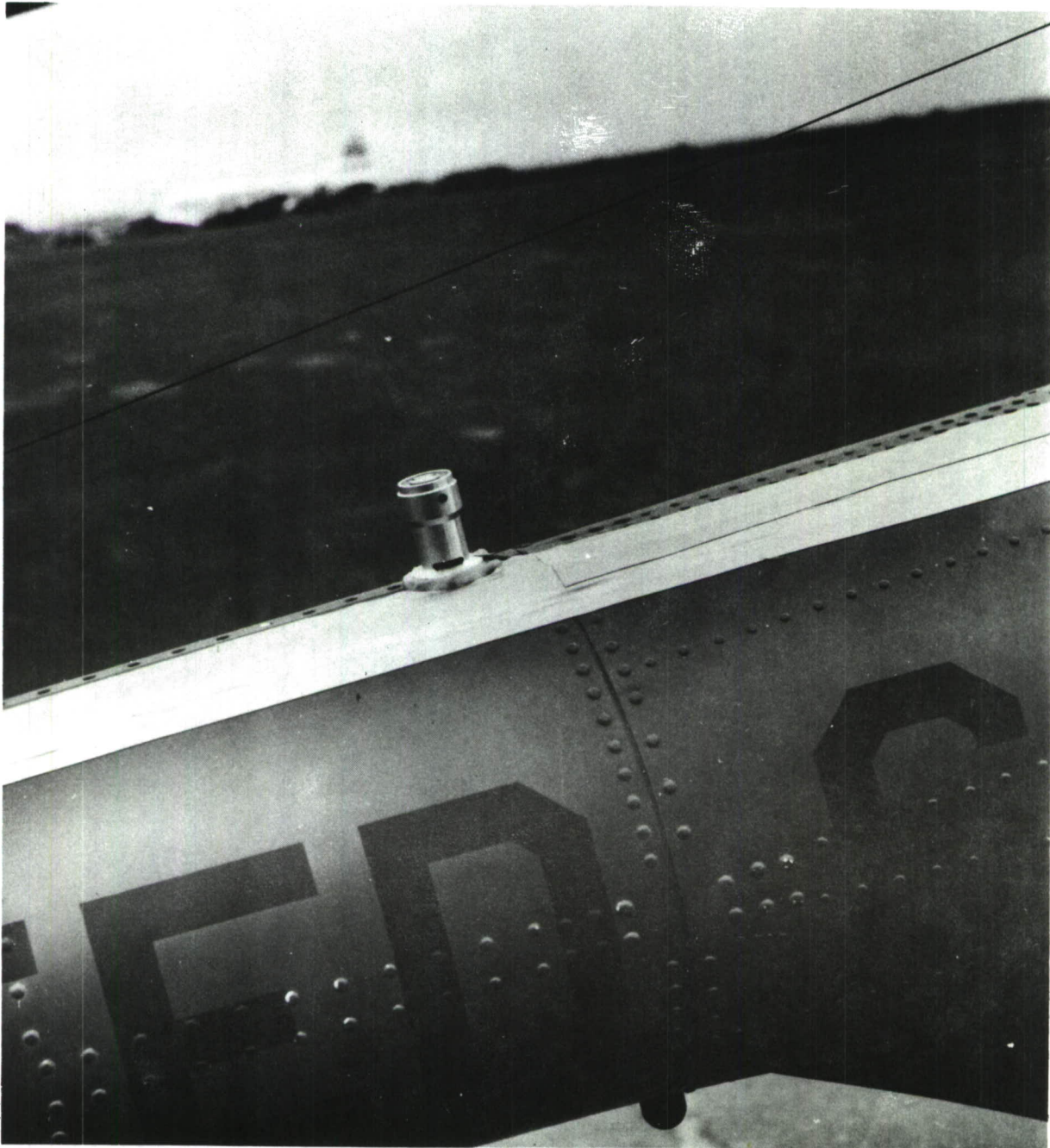
Figure 33. Microphone, Top of Fuselage, Outside, Sta. 200, PUID 71
