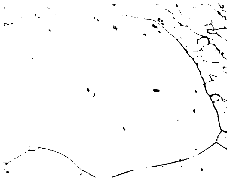
56B) 200 ppm \text{Sr}^{+2} 150X Discontinuous Grain Growth (E19038-18)
