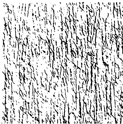
Figure 61. ManLabs Hot Forged KCl + 5 m/o KBr.
