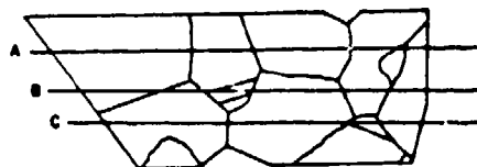
VISUAL MAPPING OF HIGH ANGLE GRAIN BOUNDARIES SHOWING LASER SCAN PATHS
