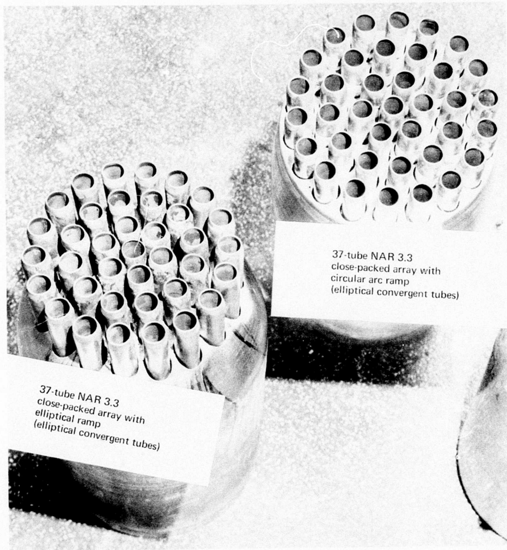
Figure 32.—Comparison of 37-Tube, 3.3 Area Ratio Nozzles
