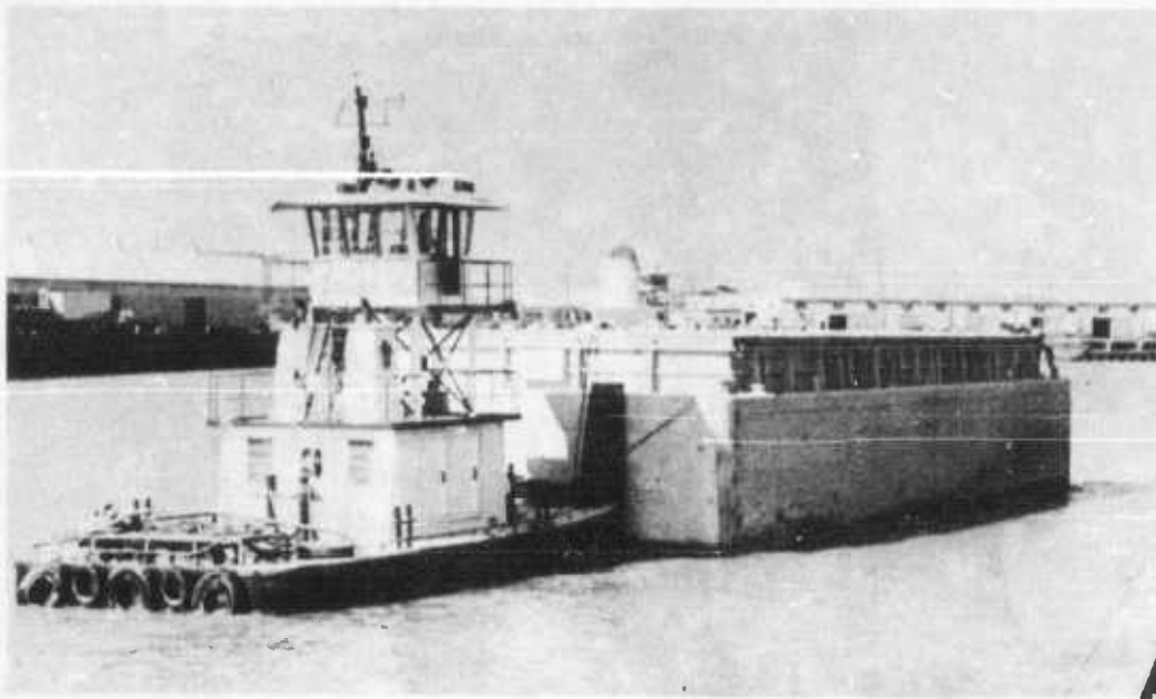
Figure 32. Berthing SEABEE Barge at Army Pier in Mobile, Alabama.
