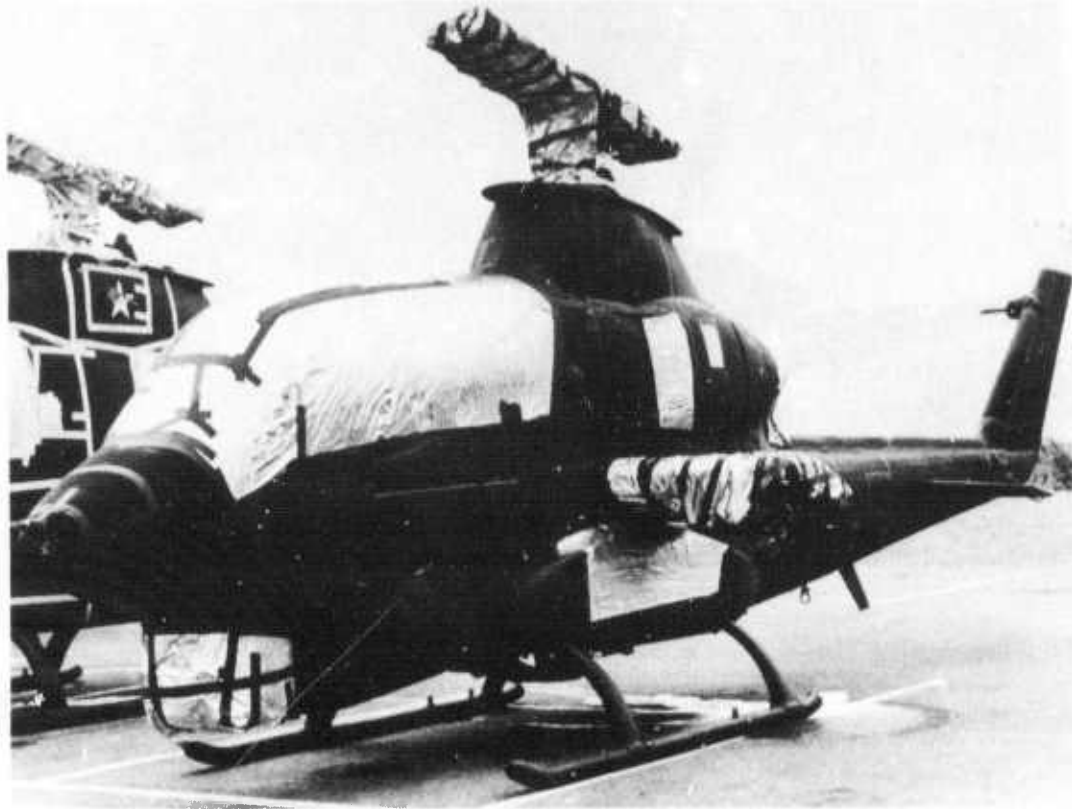
Figure 19. AH-1G Helicopter Preserved for Below Deck Sea Shipment.
