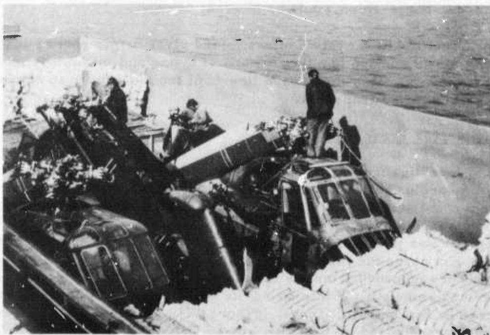
Figure 46. Three Unpreserved Civilian Helicopters Shipped in SEABEE Barge.
