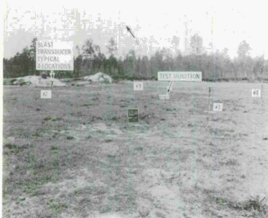
Typical Instrumentation Setup Showing Transducer Locations at 15.6 Feet - 90° Array
