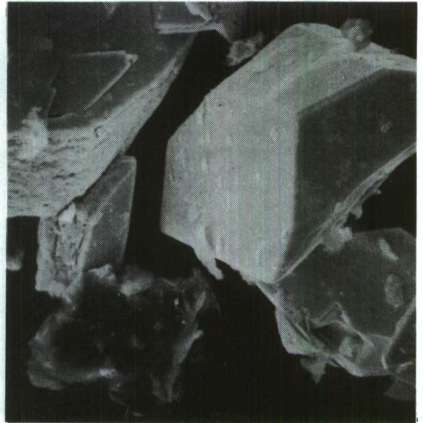
FIG. 7 RD1355 3% GRAPHITE DRY MIX. (X720)
