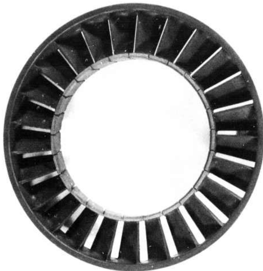
Figure 3.22 Silicon Nitride Stator After 175 Hours of Durability Testing
