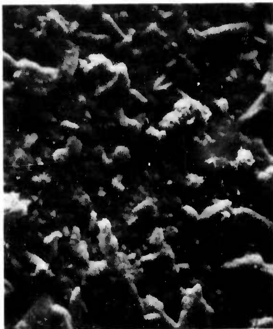
Figure 4.20 SEM of Upstream Surface of Sample 1 Norton NC 203 SiC (1000x)
