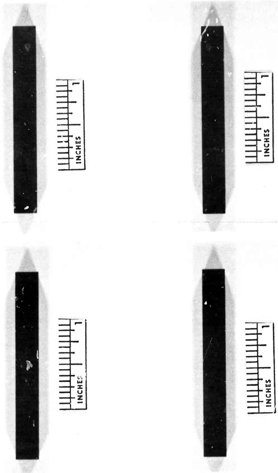
Figure 4.12 Surface Appearance of Four Sides of Norton HS-130 Hot-Pressed \text{Si}_3\text{N}_4 , Specimen 2
