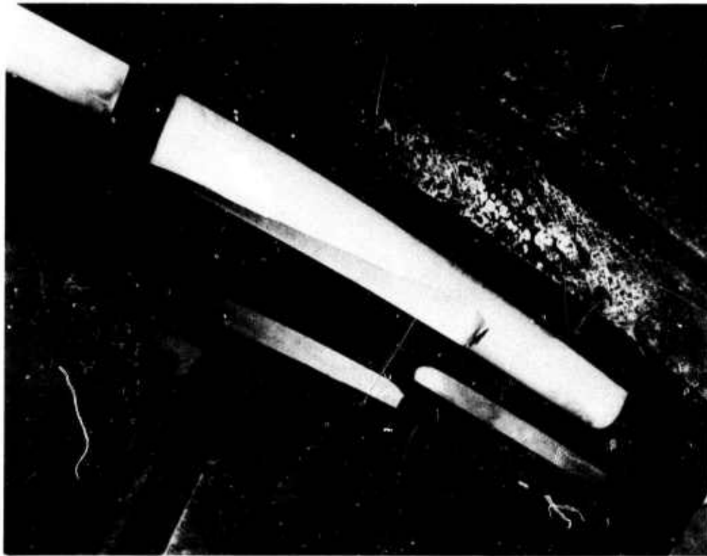
Figure 6.15 Illustration of Outer End Cap Position Shift During Static Rig Tests at 2500°F (Cycles 1-25)
