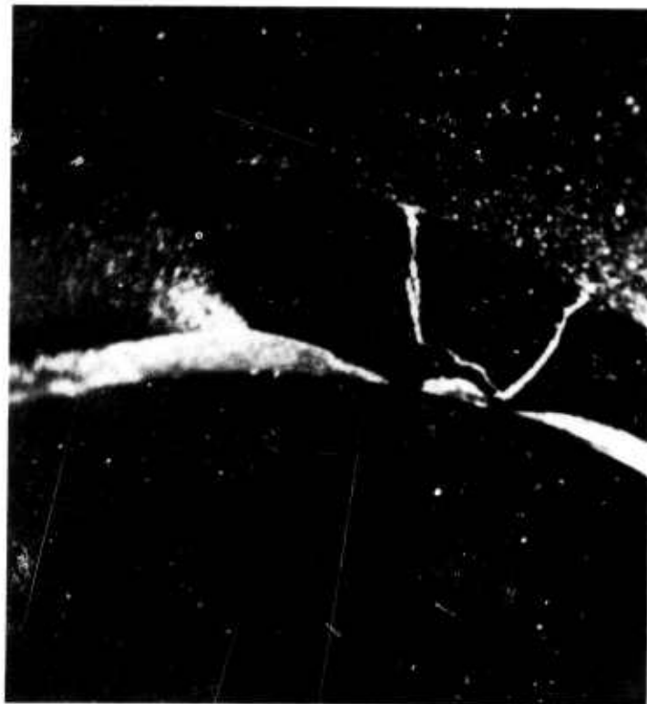
Figure 6.18 Typical Example of Chipping at the Inner End Cap-Airfoil Tenon Interface (Cycles 1-25 Static Rig Test at 2500°F)
