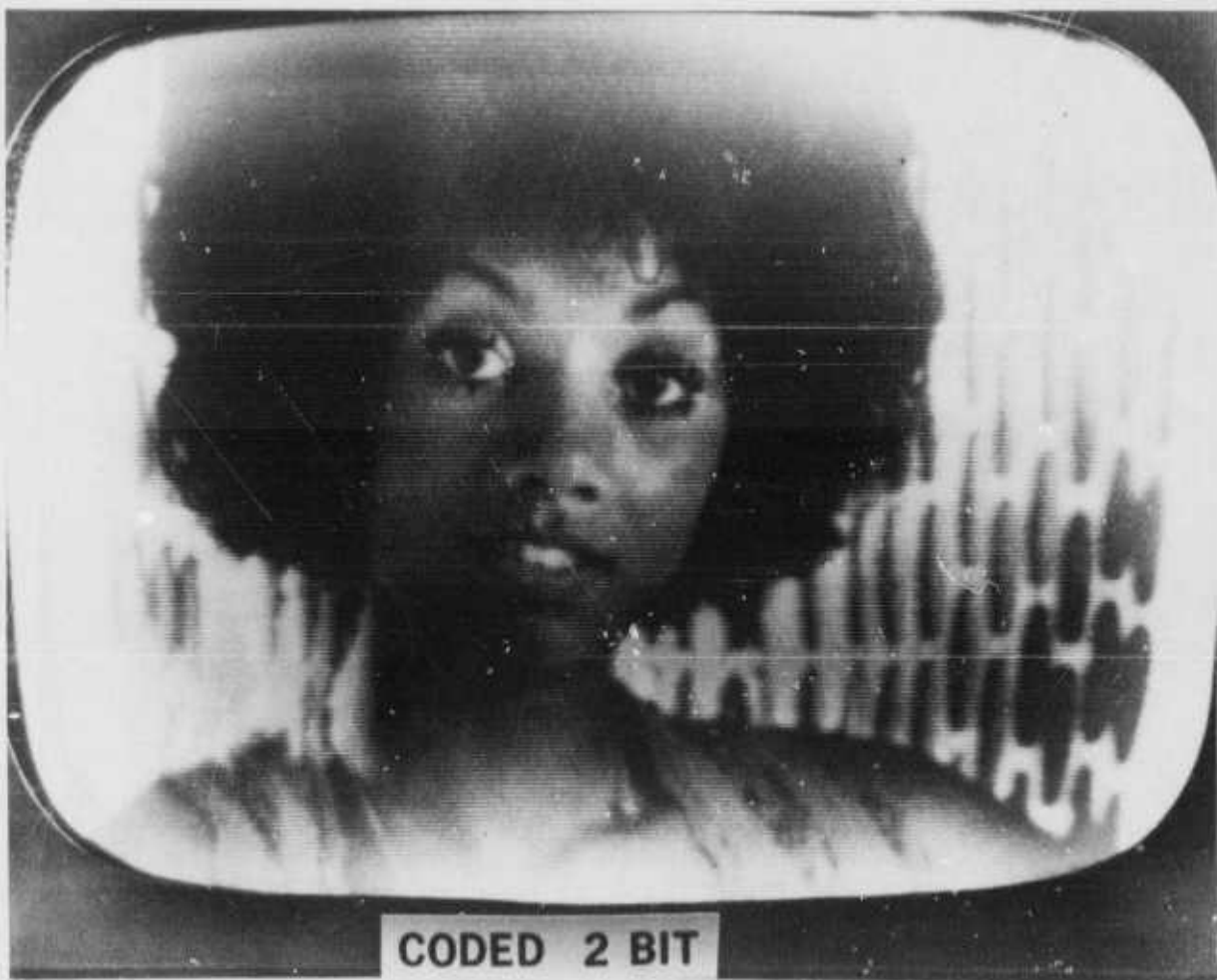
Figure 6. 2-Bit Encoded/Decoded DPCM at 10 MHz
