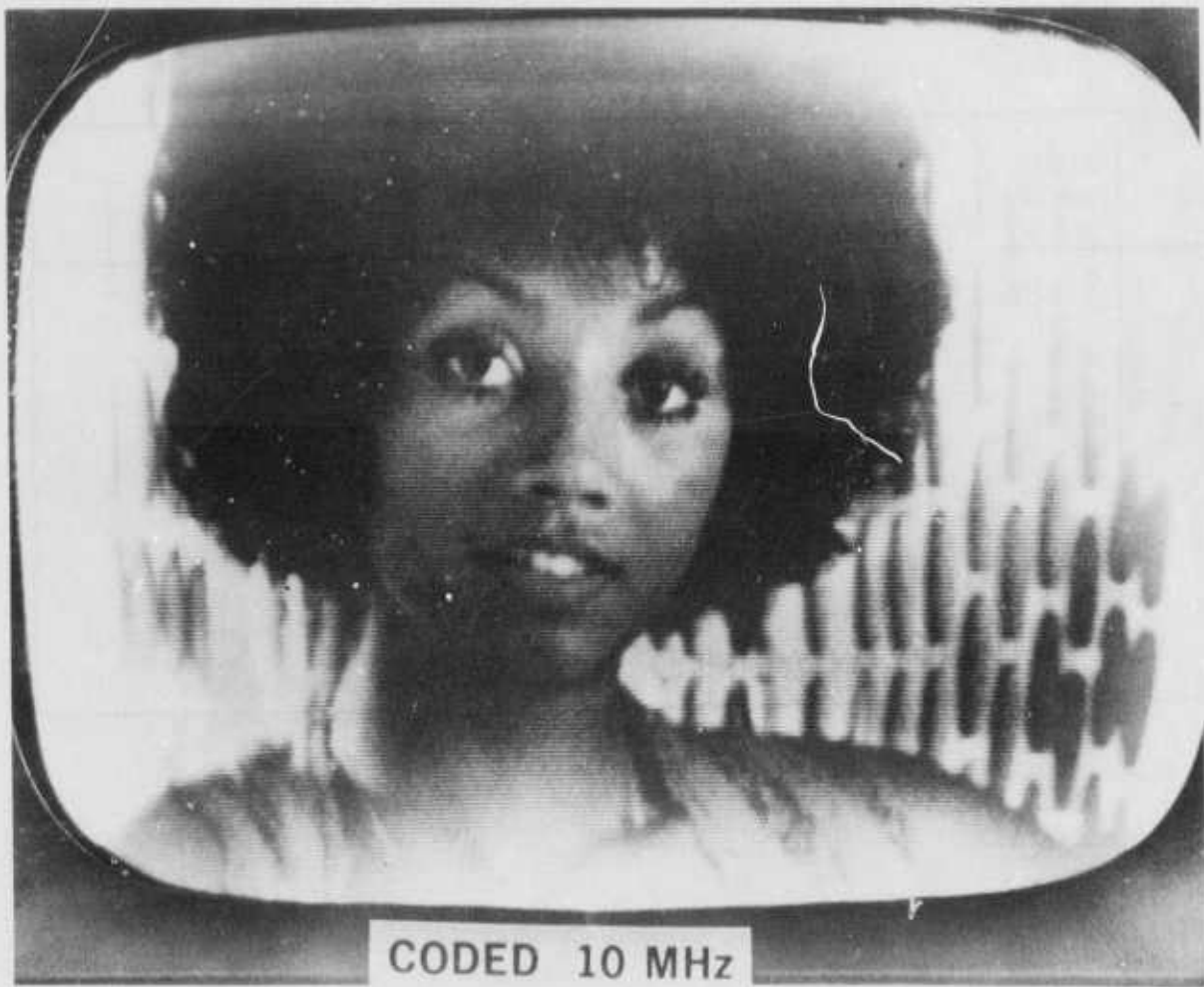
Figure 10. 3-Bit Encoded/Decoded DPCM at 10 MHz
