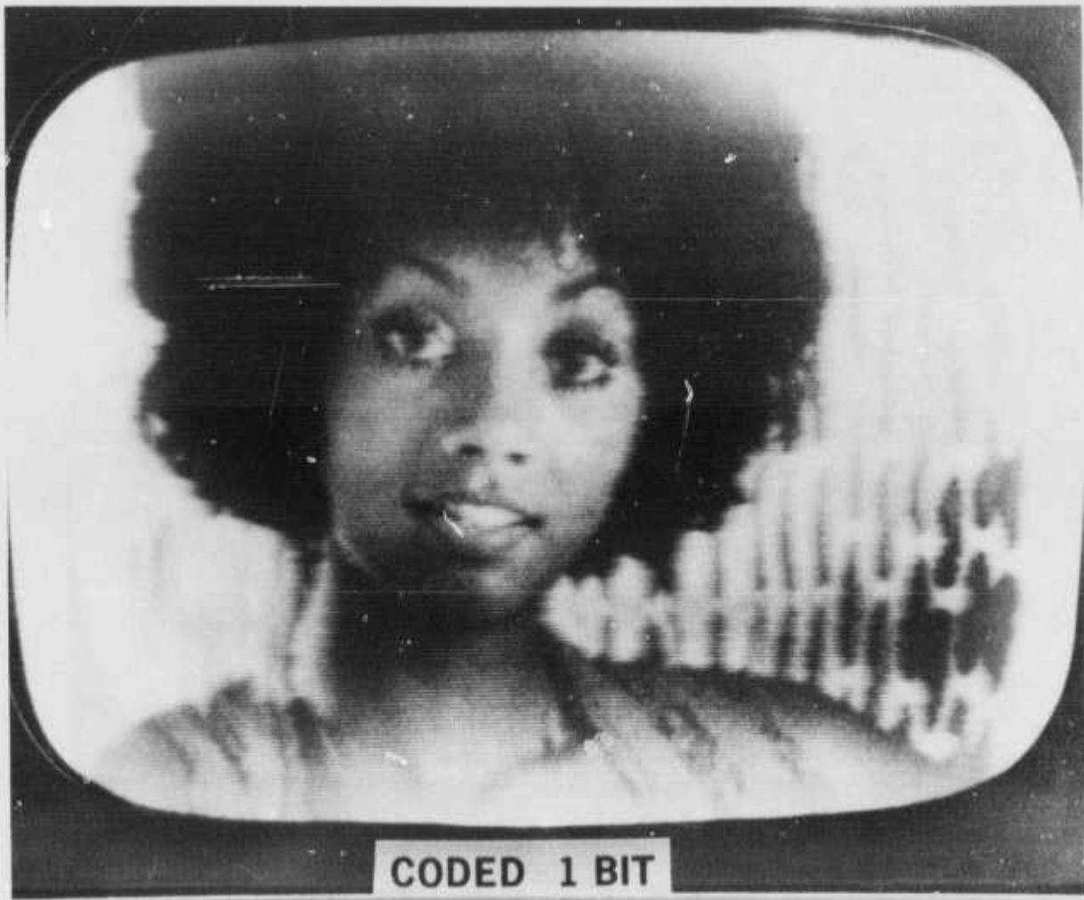
Figure 4. 1-Bit Encoded/Decoded DPCM at 10-MHz Sample Rate
