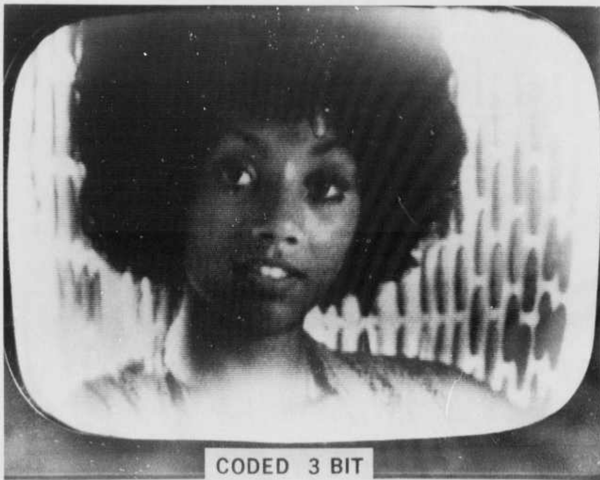
Figure 7. 3-Bit Encoded/Decoded DPCM at 10 MHz
