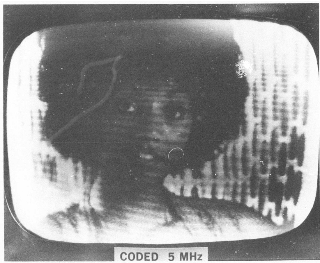
Figure 9. 3-Bit Encoded/Decoded DPCM at 5 MHz
