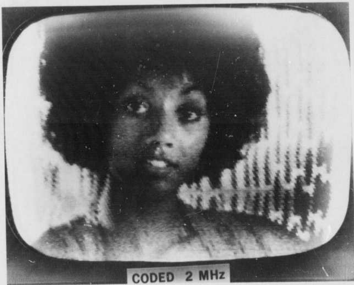
Figure 8. 3-Bit Encoded/Decoded DPCM at 2 MHz
