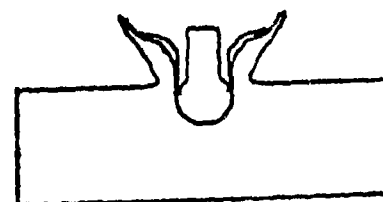
Figure A-5. Projectile/Target Configurations at Various Times for Calculation 4 ( S = 3.6 \times 10^{10} , Y_0 = 1.51 \times 10^{10} , G = 7.75 \times 10^{11} , A = 1.095 \times 10^{12} )
